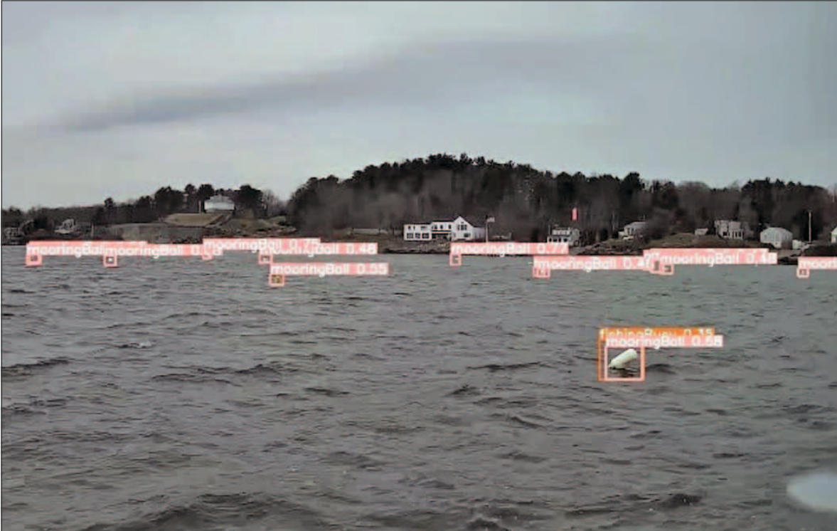
Figure ES-19. The above image from BEN's panoramic camera array was evaluated by the retrained YOLO5 algorithm, illustrating the ability to detect mooring balls and other buoys varying in range from approximately ten meters to several hundred meters in range. Notably, the image also shows a lobster pot detected as both a mooring ball and a fishing buoy. These inaccuracies can be reduced with the inclusion of more diverse images in the training data.
