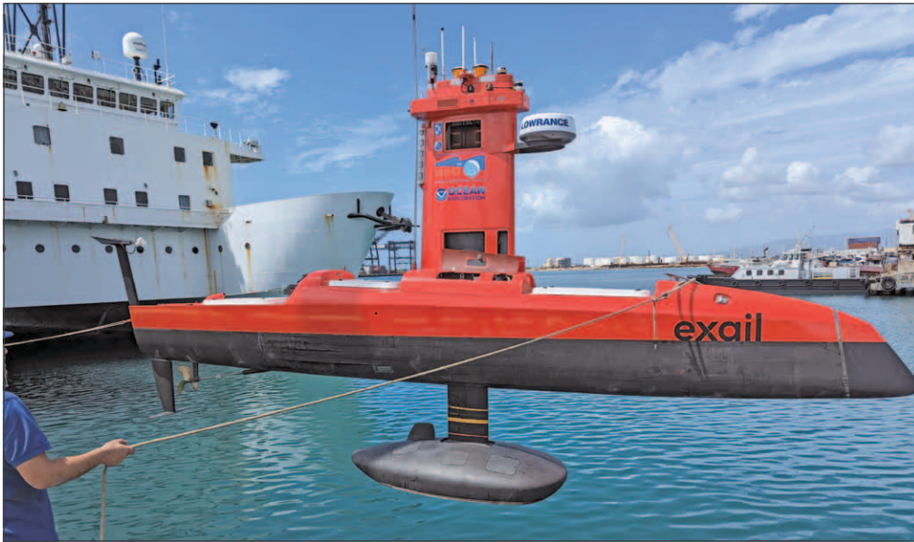
Figure ES-16. DriX-8 with new EM712 gondola and Starlink antenna during EM712 sea acceptance testing in March 2023.
