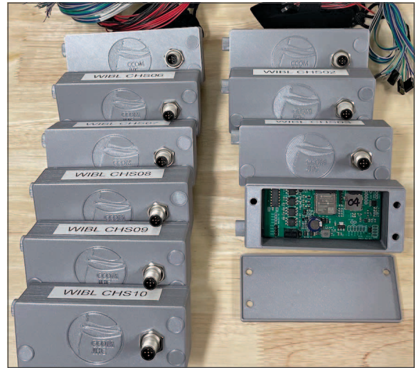
Figure ES-20. A set of 10 WIBL v2.4.1 loggers in 3D-printed boxes, along with wiring harnesses for NMEA-0183 input.
