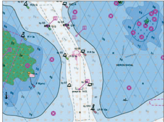
Figure ES-47. An example of S-100 compliant dot-clusters using the IHO S-100 Viewer.
