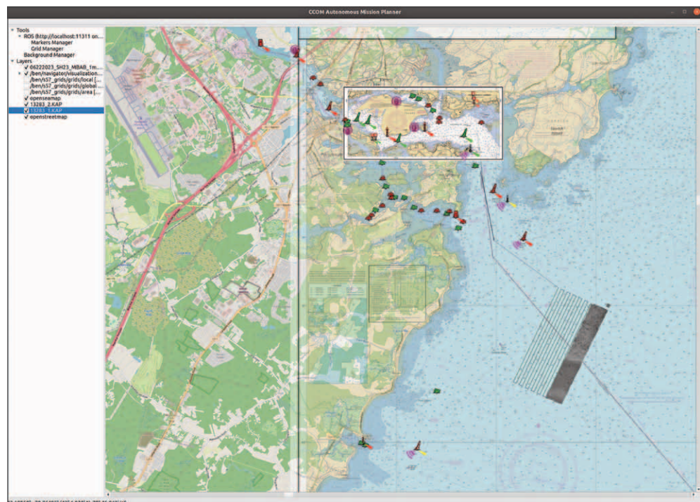
Figure ES-18. New functionality in the Center’s “CCOM Autonomous Mission Planner”, in which multiple layers of background information can be viewed with transparency simultaneously. Here previous survey data is displayed atop an OpenSeaMap rendering of the ENC, along with planned survey and transit lines.
