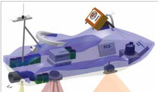
Figure 1-11. CAD drawing (right) showing the location of the MBES (peach), SBES (yellow), ADCP (red) with acoustic beam patterns on the CBASS. Also shown are the location of the POS MV IMU and PCS, onboard computers and LAN router, internal battery packs, GPS and RTK antennae, and navigational display monitor.
