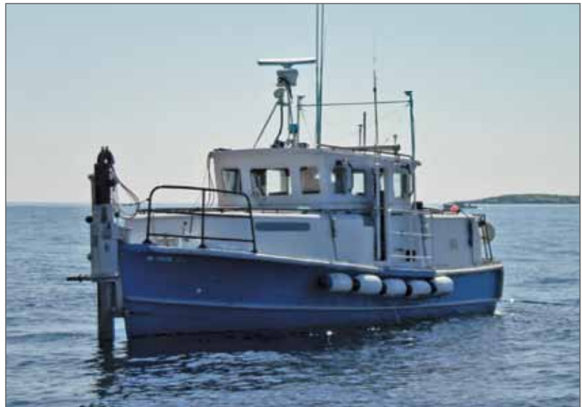
Figure 1-8. R/V Coastal Surveyor with bow ram.
