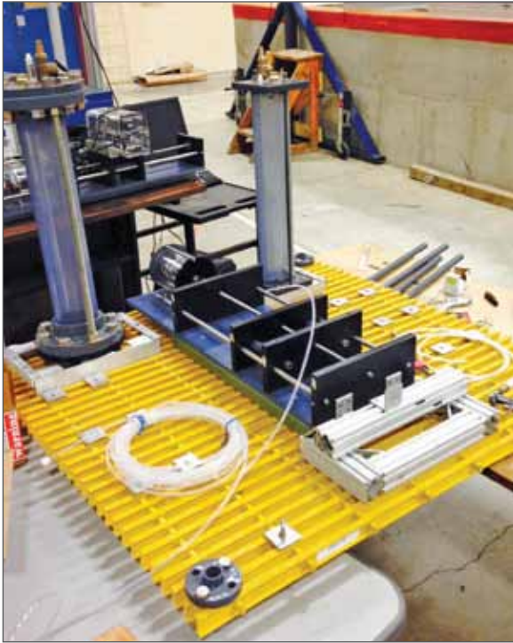
Figure 5-17. Oil droplet making apparatus with camera mount, oil tank and water tank.
