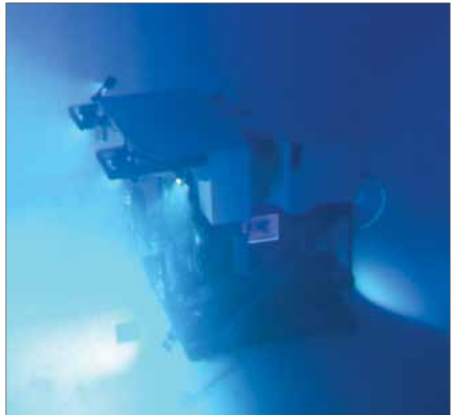
Figure 1-16. Deep Discoverer ROV being tested in the Ocean Engineering test tank at the Center.
