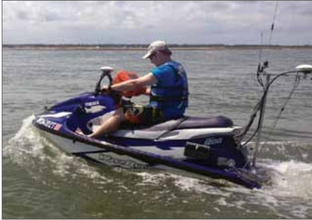
Figure 1-10. CBASS surveying in New River Inlet, NC.
