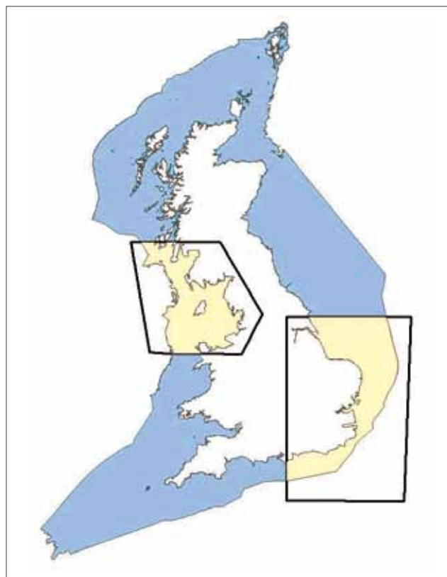
Figure 8-7. Areas to be used for re-survey priority estimation highlighted (green) against the United Kingdom survey area of responsibility (purple). The southeast area is a highly dynamic environment with high traffic density but supported by high-resolution modern surveys; the northwest area still has significant traffic density, but has only limited survey data, making for a more challenging environment.
