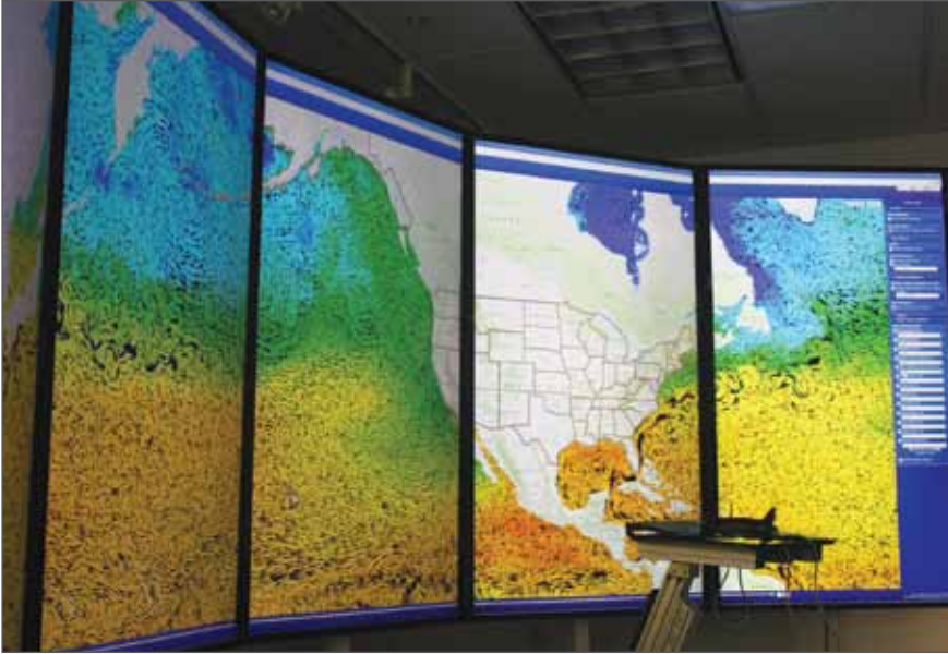
Figure 1-4. Semi-immersive, large-format tiled display.
