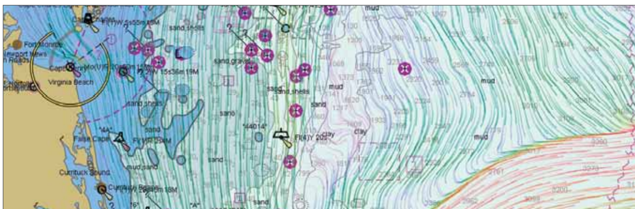
Figure 7-13. Representation of ocean currents. When animated the flow visualization minimally interferes with other chart data.
