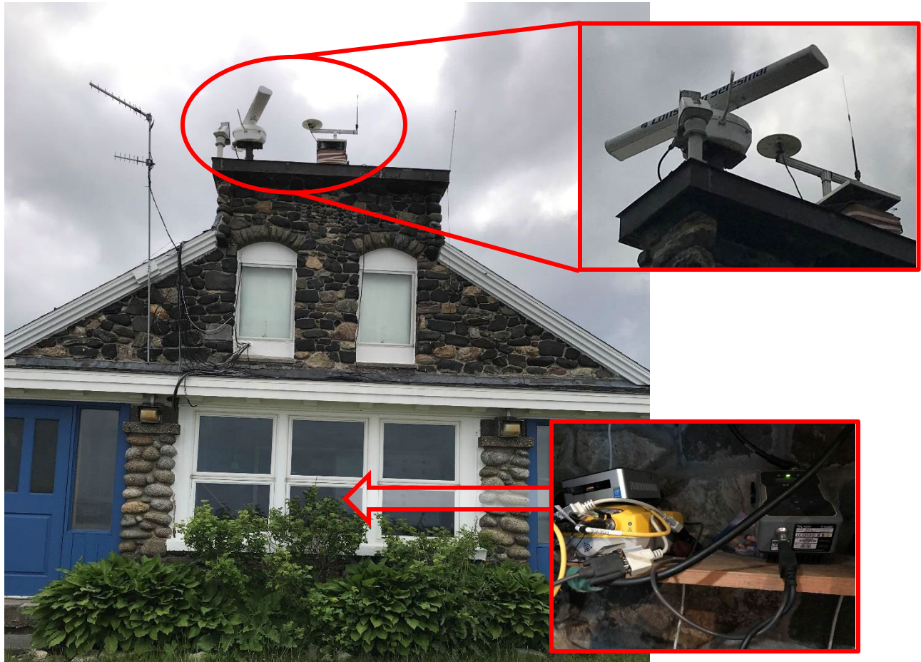
Figure 2: Instrumentation of the RTK Base Station at the Seacoast Science Center, Odiorne Park, Rye, NH
