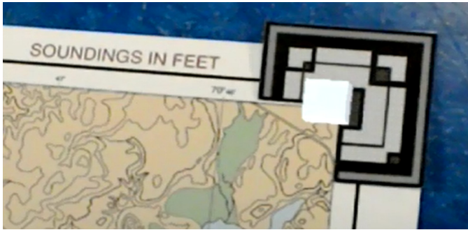
Fig. 3. A paper AR marker placed over a chart corner, with virtual anchor (white cube) that confirms it has been correctly recognized and located.
