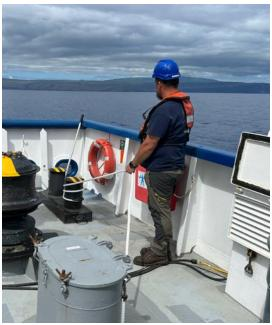
Once the monkey's fist thrown over the DriX, the ship is maneuvered forward at 1-2 knots, while line is fed through the hawsehole keeping just enough tension on the line to maintain the monkey's fist seated in the DriX towpoint. Care must be taken to anticipate ship movements so as not to inadvertently pull DriX into the ship.
