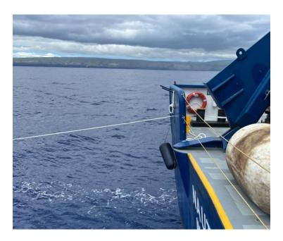
The small buoy is shackled on tow line, and if necessary to keep line from sinking into screw, positioned along the tow with a second line, allowing the buoy to ride down the towline ~30 m (100 ft) back. In the image above, the small buoy is stationed ready to deploy.
