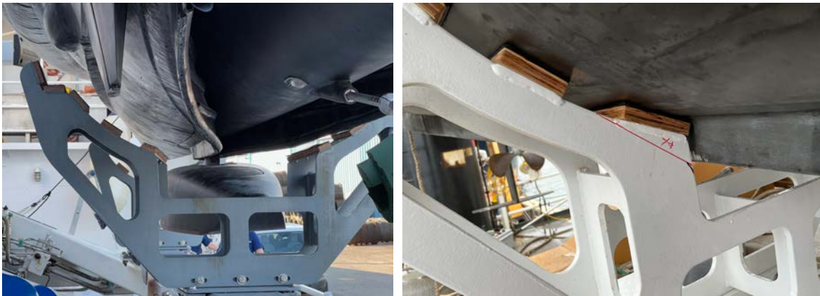
Left, the aft cradle manufactured for the Thomas Jefferson is shown with the DDS and DriX suspended above it, looking forward. On the Right, the same cradle design, this time manufactured for the Oscar Dyson with markings to illustrate material that was subsequently removed to allow self-centering of the system.
