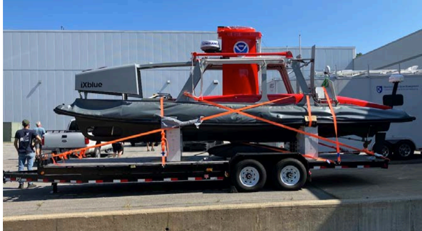
DriX 12 and DDS aboard a 28"-deck-height trailer, and antennas removed to meet Department of Transportation road height requirements (total height approx. 10ft, 8").
