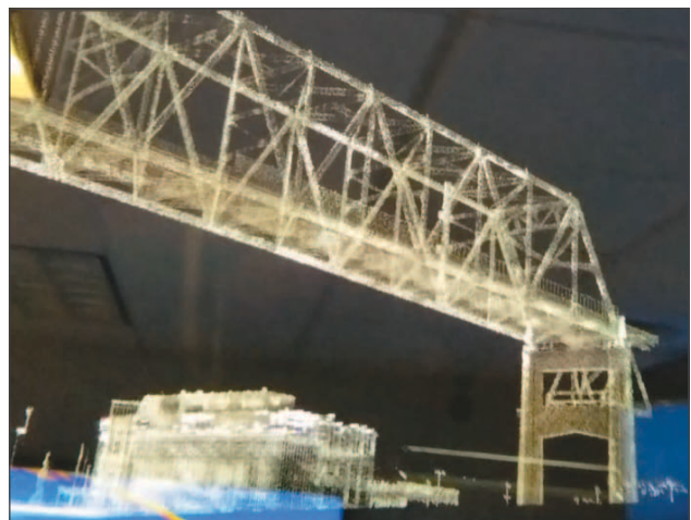
Figure 40-1. Point cloud of the Crescent City Bridge as seen through the lens of the Nreal Light AR glasses. Point density had to be reduced to render at interactive speeds.
