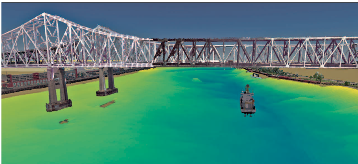
Figure 32-6. High-resolution S-102 bathymetry as a 3D surface, with user-uploaded 3D model of ship.
