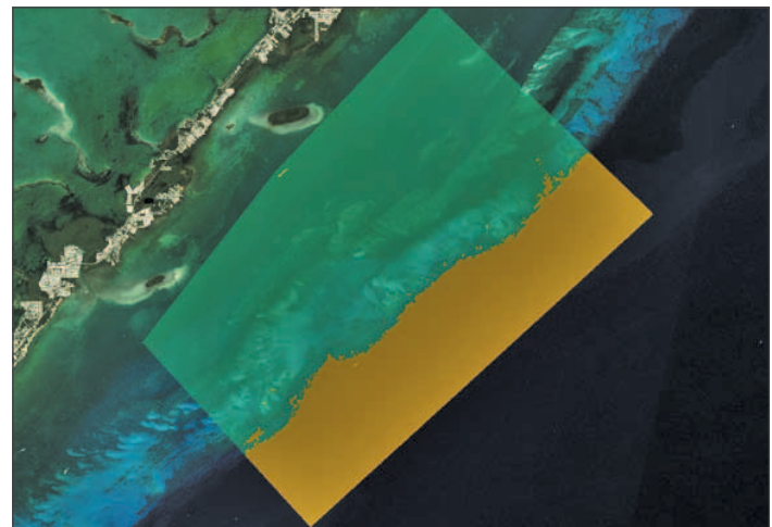
Figure 29-5. SDB bathymetric grid used for auto-segmentation of true vs. false bathymetry.
