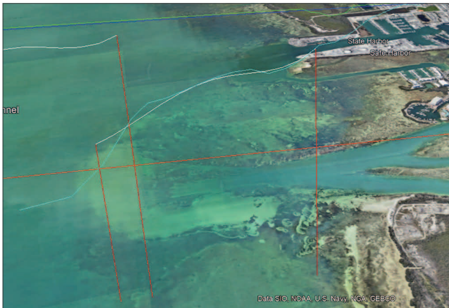
Figure 25-3. Example of bathymetry derived from ICESat-2 (cyan line) and NOAA airborne Lidar (white line). The green line at the top is ocean surface, the red horizontal line is 5m depth, and the bottom of the red vertical lines indicate the location of the track on the Earth's surface.
