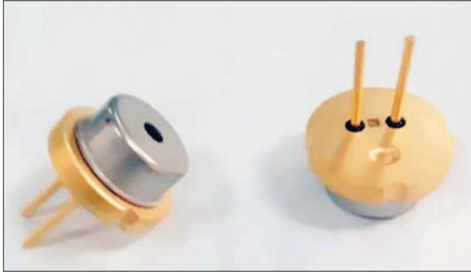
Figure 22-1. 520 nm laser diode NGD7475. Manufactured by Nichia Corporation, Japan.
