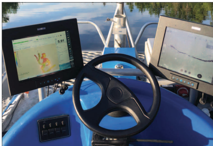
Figure I-12. System displays on JHC Zego Boat.
