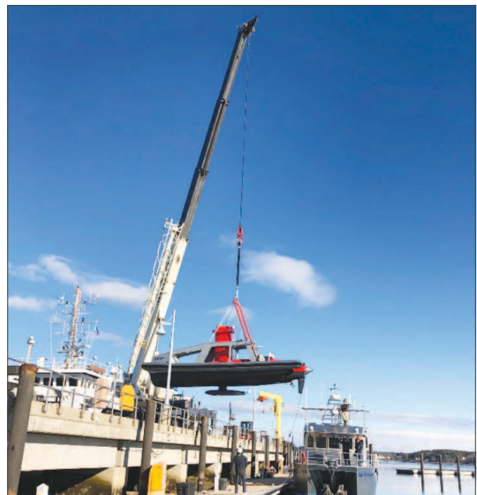
Figure I-15. Exail (iXblue) DriX autonomous surface vehicle being lowered into the water in its Launch and Recovery System.
