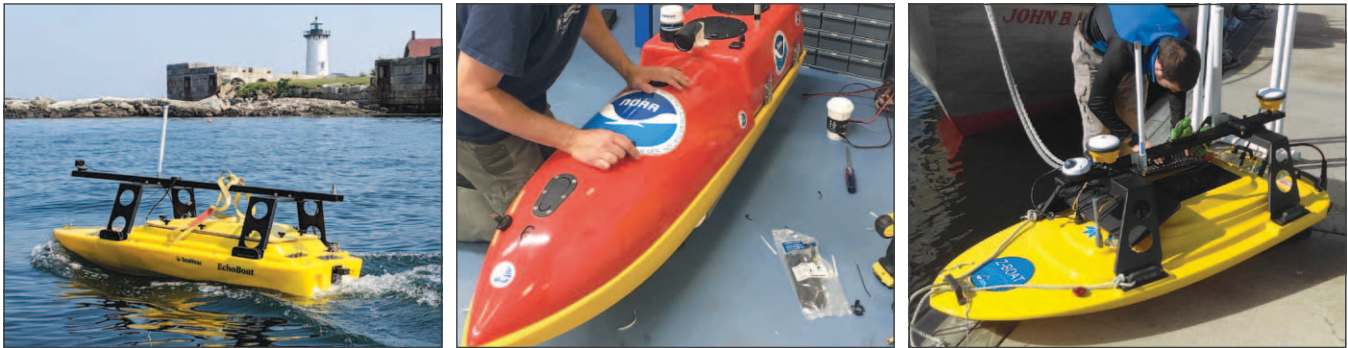
Figure I-14. Seafloor Systems’ “Echoboat” (upper), Hydronalix “Emily Boat” (middle,) and Teledyne Oceansciences’ “Z-Boat,” small autonomous surface vessels used by the Center to develop autonomous command and control algorithms.
