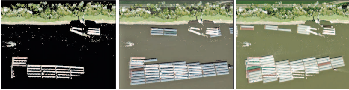
Figure 39-2. (left) view of lidar in editor, showing uncharted barge moorings, (middle, right) views of lidar with satellite photos reference maps from different times, showing there are usually barges moored here, though not always the same number of barges.
