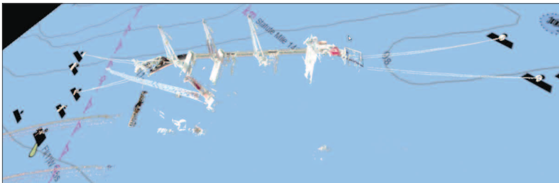
Figure 39-1. Mississippi River lidar data in the editor, with an ENC reference map indicating the mooring buoys that should be preserved while editing out the ship and the mooring lines.
