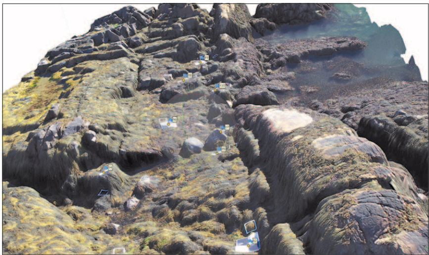
Figure 23-4. Ground level view of 3D Model: Ground level view of 3D model with draped imagery showing one of the intertidal zone sites. Note the high resolution and low visible distortion due to the high local accuracy of the model whose geometry is constrained by accurately positioned GCPs.
