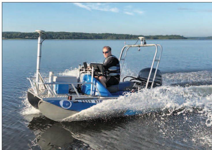
Figure I-11. The JHC Zego Boat, a highly maneuverable and stable twin-hulled catamaran that is being outfitted into a state-of-the-art shallow water survey vessel with MBES, SBES, and ADCP capabilities.
