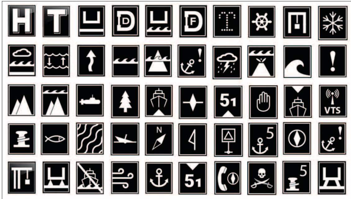
Figure 37-3. Preliminary symbols for the new feature types in S-126, S-127, and S-131, built for 3D interactive web-based applications.
