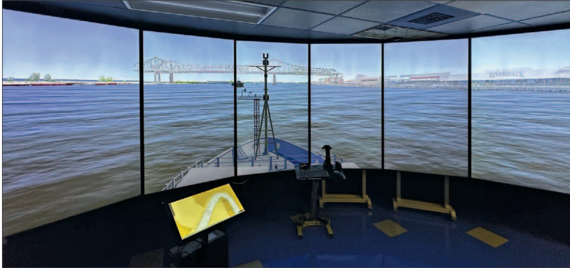
Figure 32-7. The visualization lab's semi-immersive tiled display running a head-tracked bridge simulator with accessory monitor that can display ECDIS (reflecting virtual ship's position/orientation) and augmented camera feeds generated from a virtual camera.
