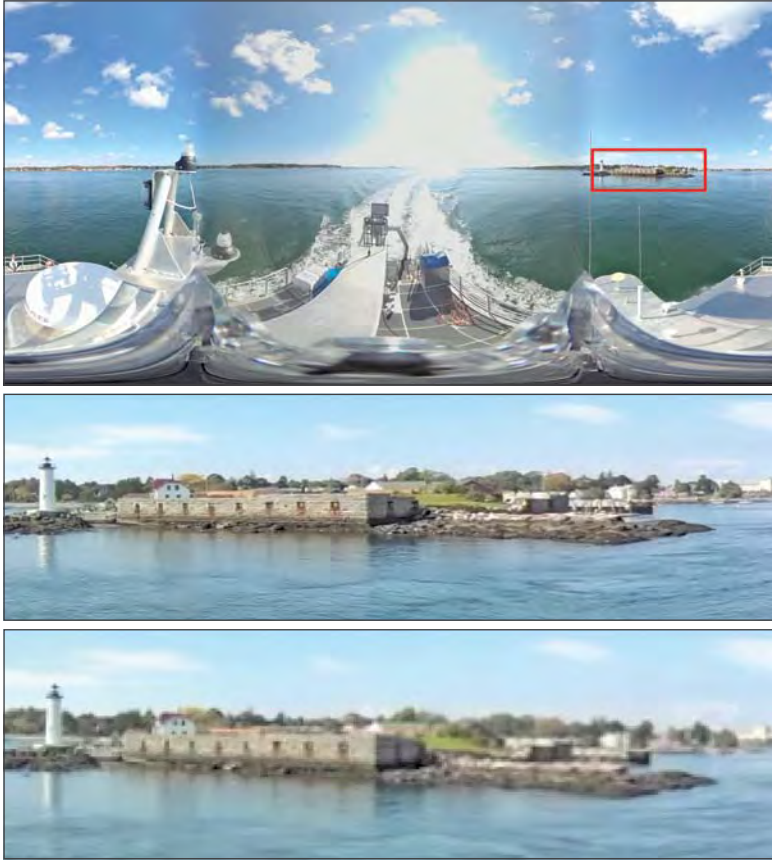
Figure ES-14. (top) Original 360° video frame, and location of example region; (middle) example region visual quality using packing; (bottom) example region visual quality using traditional scaling. The video size is the same in each.
