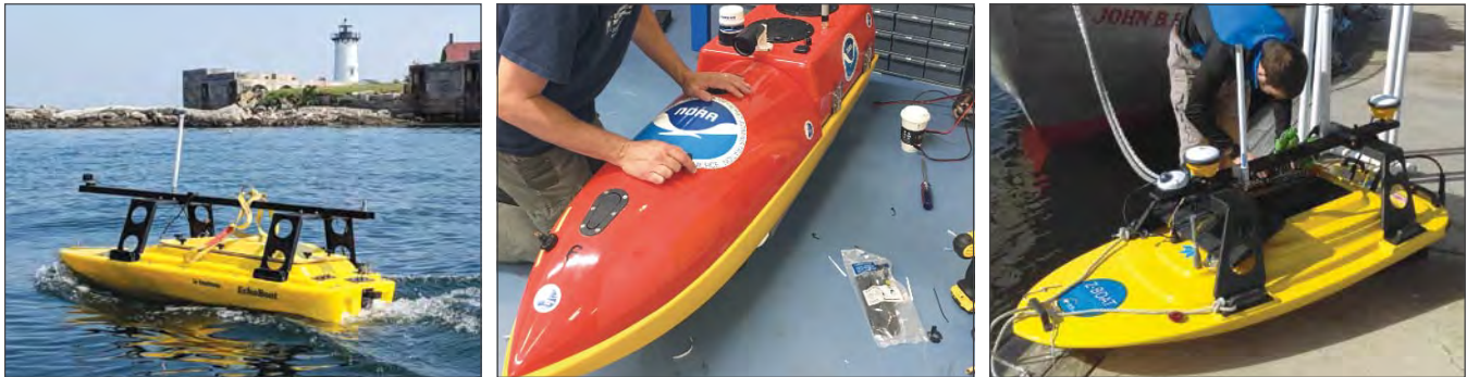
Figure I-15. Small autonomous surface vessels used by the Center to develop autonomous command and control algorithms: Seafloor Systems’ “Echoboat” (left), Hydronalix “Emily Boat” (center), and Teledyne Oceansciences’ “Z-Boat” (right).
