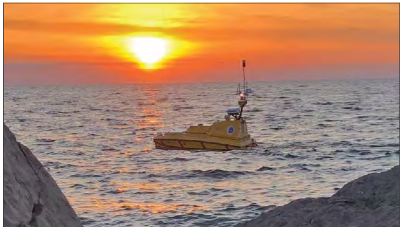
Figure I-14. BEN (the Bathymetric Explorer and Navigator), a CWorker-4 model vehicle, operating under an eclipse while mapping in Lake Michigan's Thunder Bay Marine Sanctuary.
