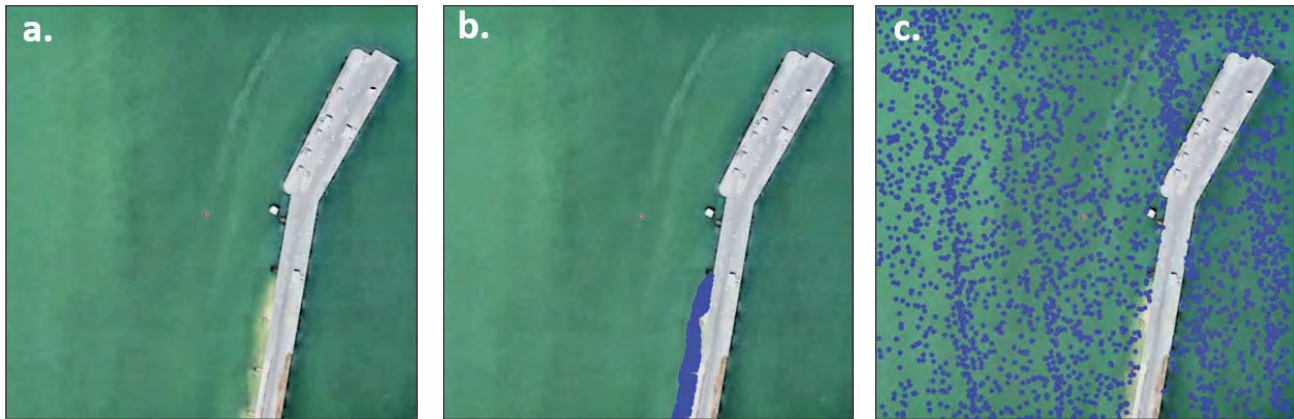
Figure 16-5. Example of tile on which infrastructure is present. a. GoogleEarth™ imagery. b. NOAA classification Bathymetry soundings (blue). c. CHRT-ML 1.0 Bathymetry soundings (blue). (For 2b and 2c, a random sub-sample of soundings is displayed to improve interpretation.)
