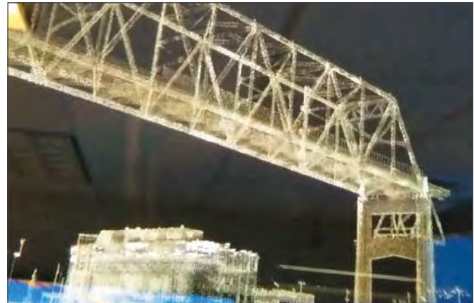
Figure ES-30. Point cloud of the Crescent City Bridge as seen through the lens of the Nreal Light AR glasses. Point density had to be reduced to render at interactive speeds.
