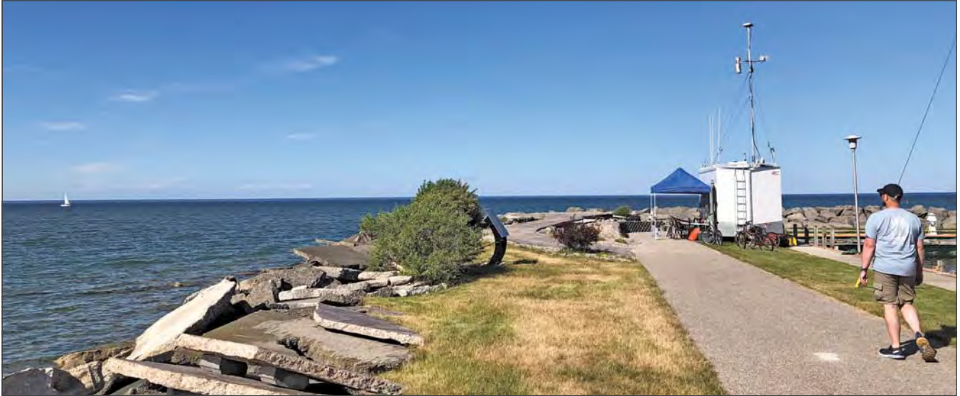
Figure 9-3. Here the Center's ASV Control Van with antenna array for multiple redundant telemetry systems is depicted. Clint Marcus, graduate student and NOAA physical scientist in the foreground.
