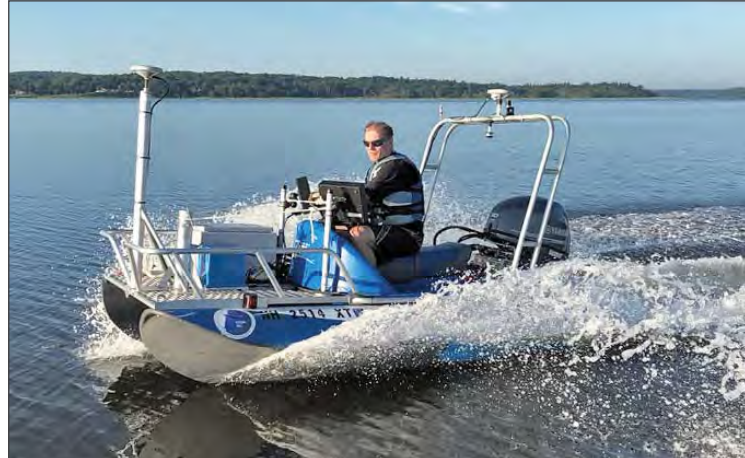
Figure I-12. The JHC Zego Boat, a highly maneuverable and stable twin-hulled catamaran that is being outfitted into a state-of-the-art shallow water survey vessel with MBES, SBES, and ADCP capabilities.
