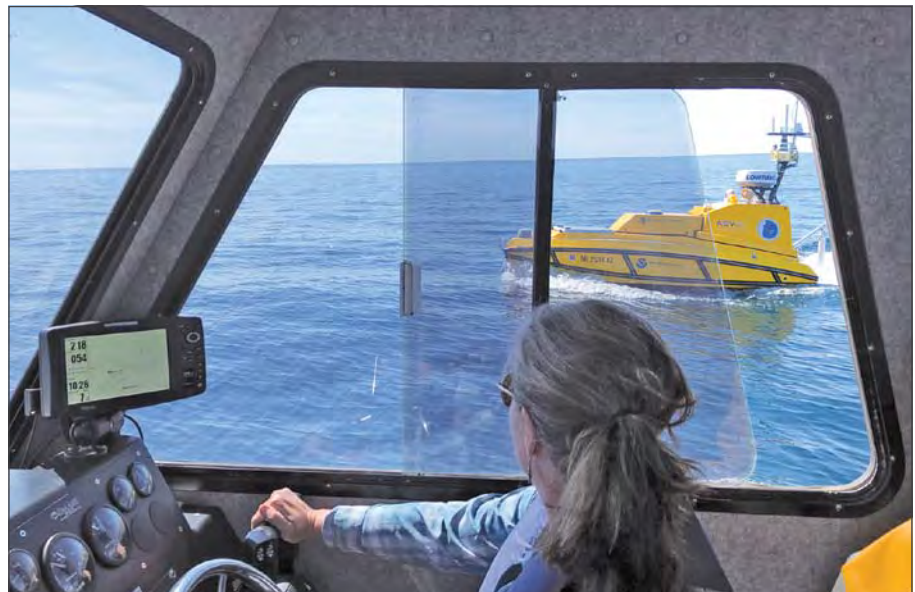
Figure ES-13. ASV BEN being chaperoned by Stephanie Gandulla (NOAA Sanctuaries) and a remote piloting team aboard NOAA Launch 301. In this mode, the coverage can be doubled and the launch used to extend the telemetry range achievable from shore.
