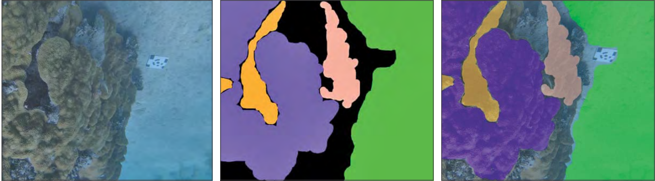
Figure 39-4. From left: original video frame; SfM model with annotation textures—rendered from same camera viewpoint; and composite of video frame and annotation output for training AI/ML.
