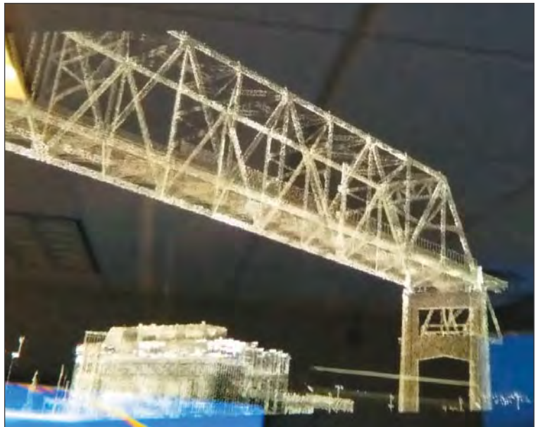
Figure 40-2. Point cloud of the Crescent City Bridge as seen through the lens of the Nreal Light AR glasses. Point density had to be reduced to render at interactive speeds.
