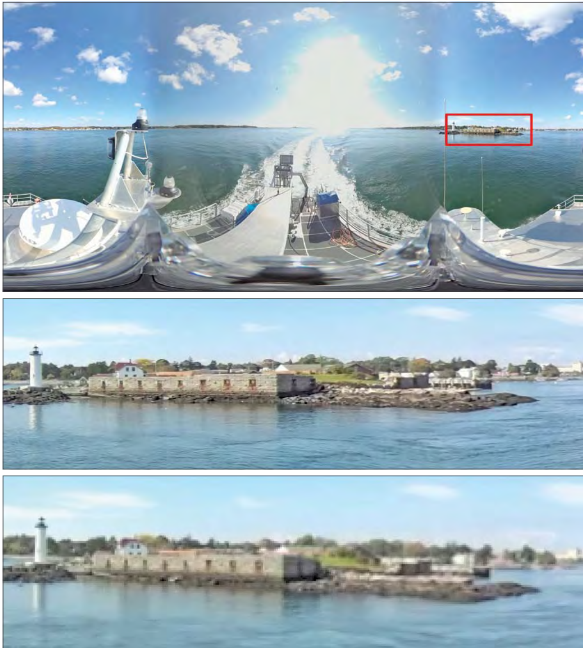
Figure 10-2. (top) Original 360° video frame and location of example region; (middle) example region visual quality using packing; (bottom) example region visual quality using traditional scaling. The video size is the same in each example.
