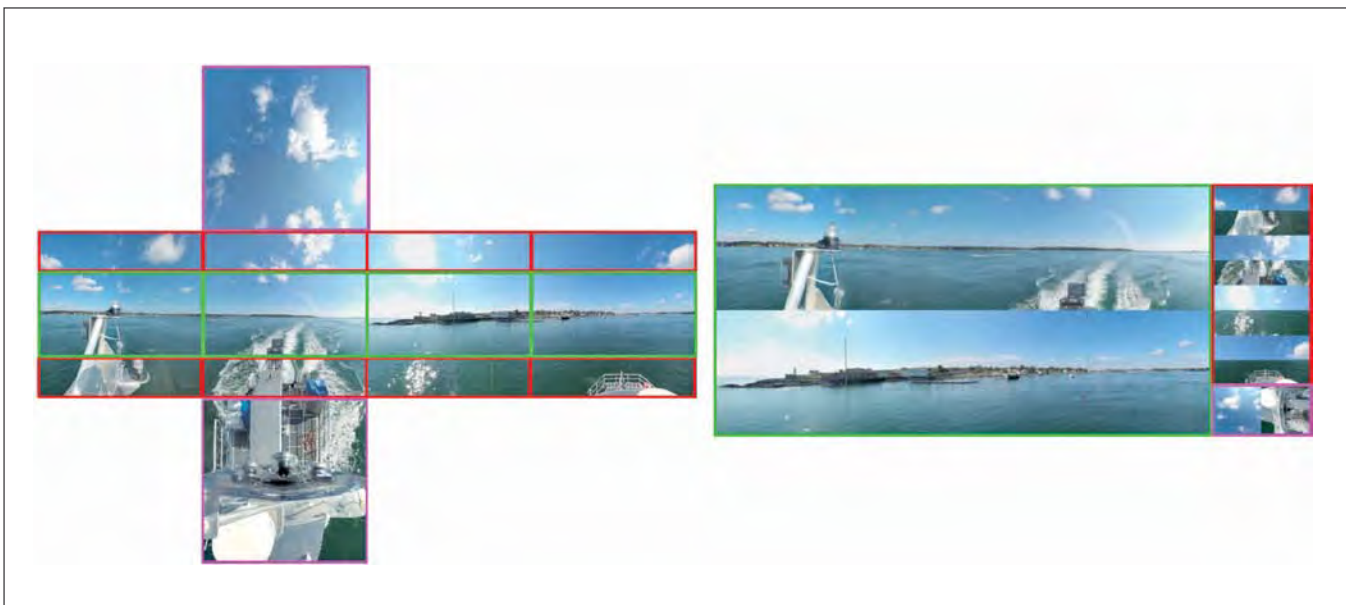
Figure 10-1 A 360° cube map video frame in original, unpacked format (left), and packed format (right). The green areas around the horizon are preserved at full resolution, the red areas above and below are scaled down to 40% resolution, and the pink areas of sky and boat deck are sent at only 10% resolution.
