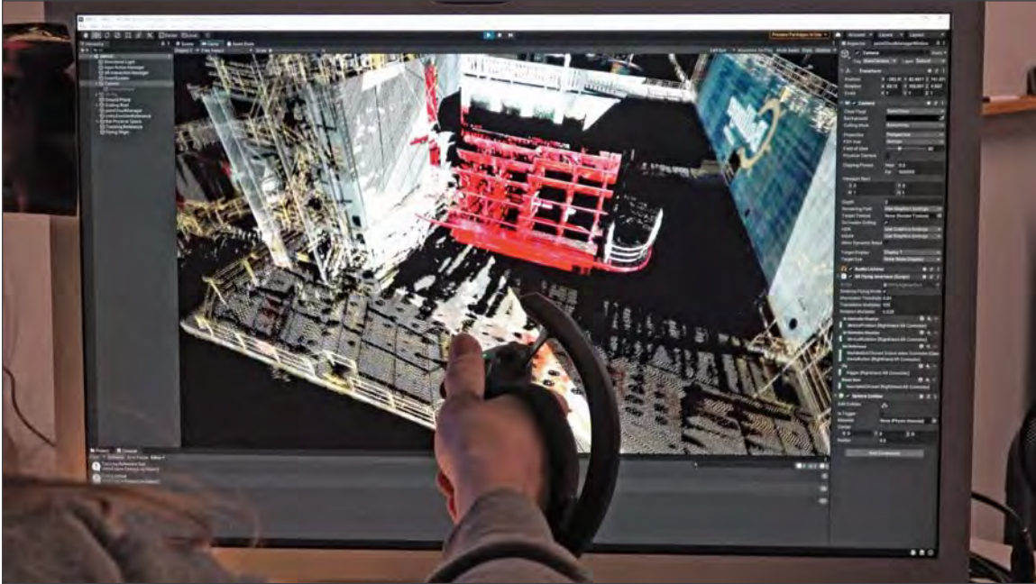
Figure 36-1. A Valve Index tracked controller is used to navigate around a 3D point cloud loaded into Unity with the point cloud plugin and the 3D flight script in 'Desktop' mode.
