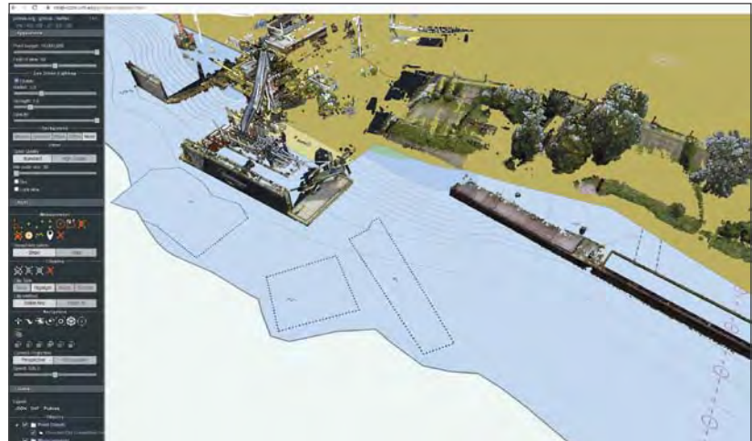
Figure 32-13. Example view of the web-based interface, showing color lidar point clouds drawn over NOAA ENCs.
