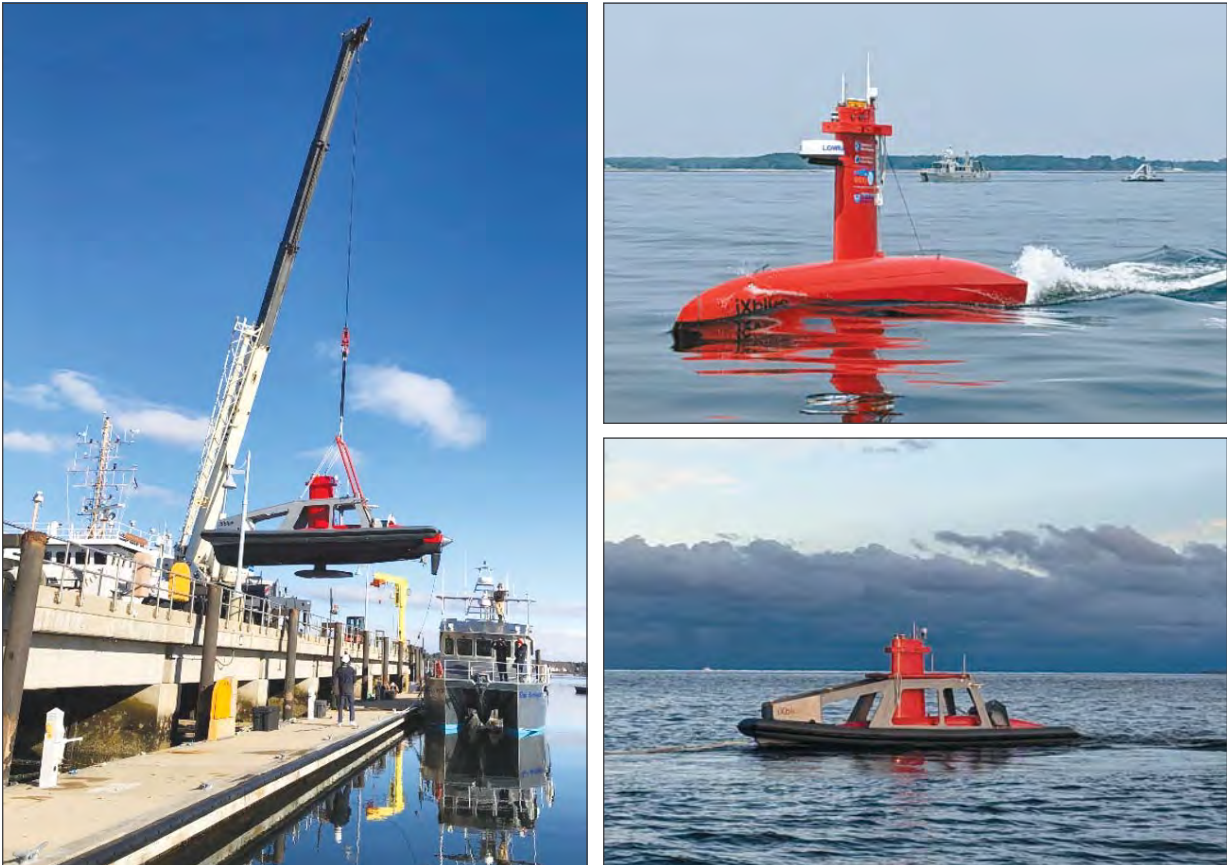
Figure I-17. Clockwise from left: the iXblue DriX autonomous surface vehicle in its Launch and Recovery System (LARS) being lowered into the water at the UNH Marine Pier in New Castle, NH; steaming through Portsmouth Harbor, NH with the R/V Gulf Surveyor and the LARS in the background; and in the LARS under a dramatic sky in Portsmouth Harbor, NH.
