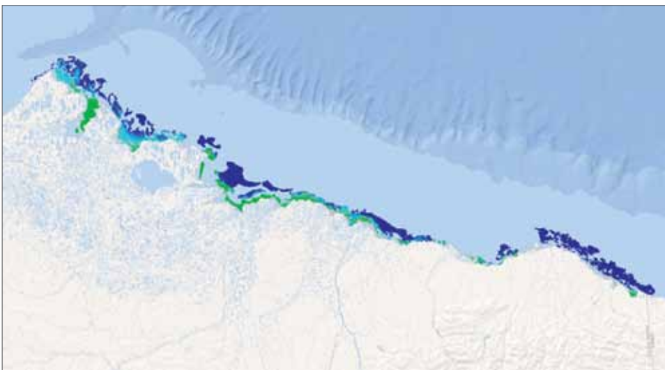
Figure ES-7. Shallow-water bathymetry derived offshore of the North Slope of Alaska using Landsat 7 (1999-2003) and Landsat 8 (2013) imagery.
