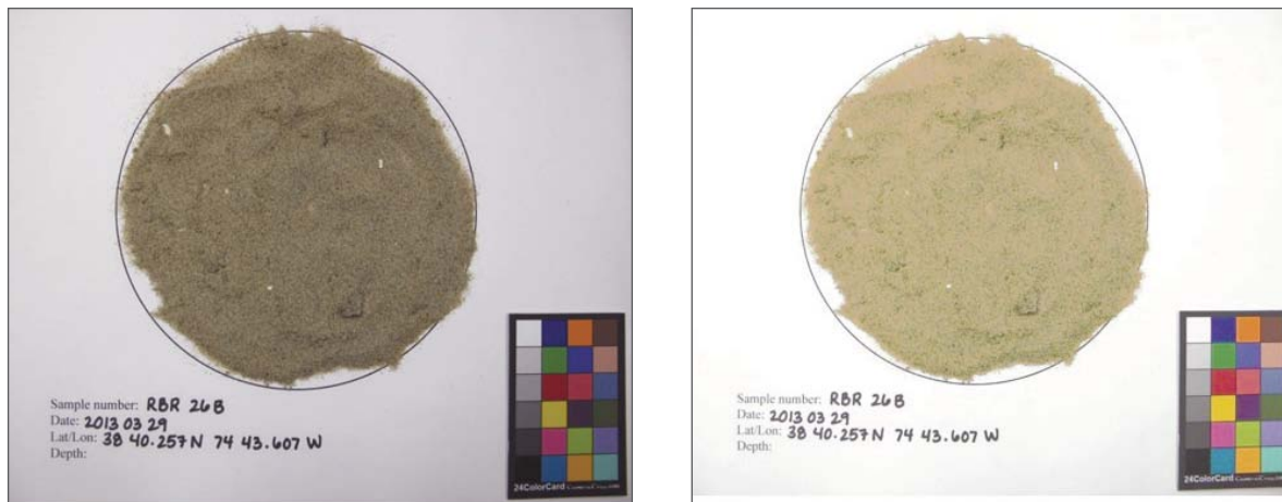
Figure 5-8. Knowledge of 24 true colors and their appearance in the image allows for solution of coefficients for 3D warping (in RGB space). Original image of sea floor sediment sample (left) and image with warped colors based on knowledge of MacBeth color table.
