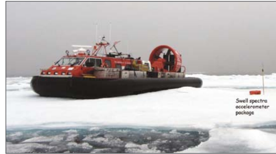
Figure 1-11. R/H Sabvabaa measuring wave swell spectra on Yermak Plateau.
