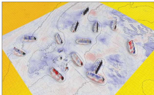
Figure 7-4. Animated dynamic bathymetry at the Redbird reef site generated within VTT4D from five overlapping survey missions. Red areas are experiencing erosion, blue areas are deposition.
