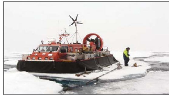
Figure 1-13. R/H Sabvabaa with 7 m-long dart corer. Note the hovercraft’s ability to operate even on very small floe.
