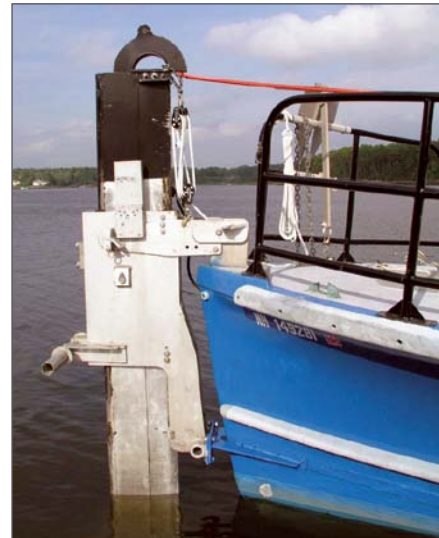
Figure 1-7. R/V Coastal Surveyor's bow ram lowered.
