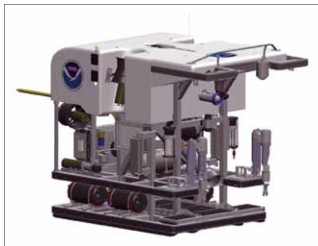
Figure 1-14. New 6000 m ROV being developed by OER at the Center.
