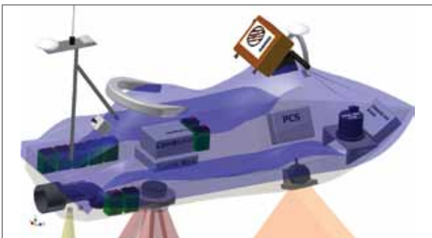
Figure ES-2. Scaled CAD drawing showing the location of the MBES (peach), SBES (yellow), ADCP (red) with acoustic beam patterns on the CBASS.
