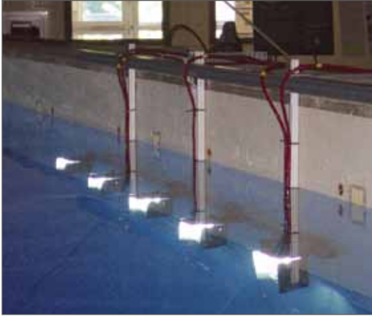
Figure 3-14. Light wall that produces an illumination that simulates natural daylight and diffuse attenuation co-efficient plot of the Cener's tank environment calculated from the irradiance measurements overlaid on the Jerlov plots.
