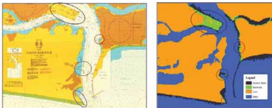
Figure 4-11. (Left) Admiralty Chart of Lagos Harbor. (Right) Classification of man-made features over Lagos Harbor, Nigeria based on satellite imagery (Landsat 7). Key features in the harbor are circled in both images.
