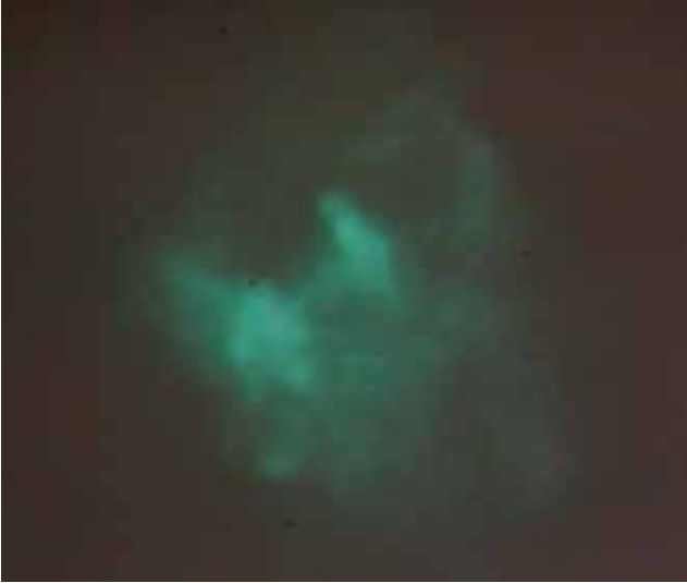
Figure 3-10. An example of a laser beam pattern (cross section) collected underwater with a wind-driven surface (wind speed of 4 m/s).
