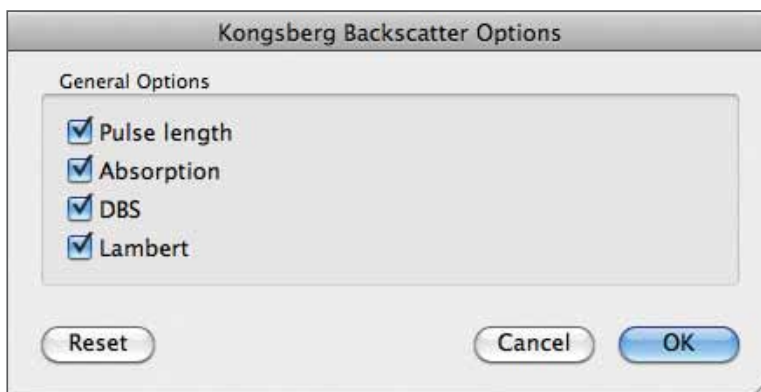
Figure 4-16. Example plug-in configuration interface implemented for the Kongsberg Backscatter processing stage. This dialog allows for fine-grained control over the corrections that are applied in processing.
