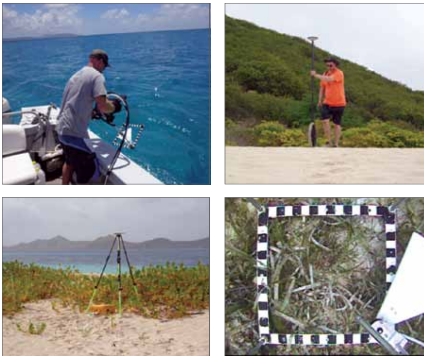
Figure 3-11. Field data acquisition in the USVI. Clockwise from top left: deploying underwater spectrometer and video camera; GPS transects; underwater video imagery of a seagrass site; and GPS basestation. In the bottom right image, the underwater calibration panel for the spectrometer can be seen. This device enables efficient and reliable acquisition of seafloor reflectance spectra.
