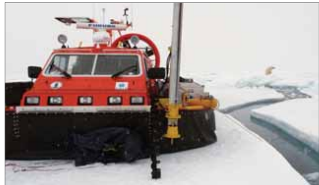
Figure 1-6. R/H Sabvabaa deployed on the ice with ice drill. Note the polar bear observing operations.
