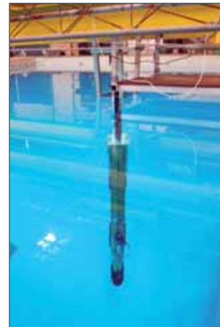
Figure 3-4. Gavia AUV mounted vertically for calibration of the Geoaoustics Geoswath
