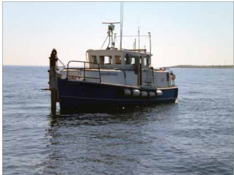
Figure 1-4. R/V Coastal Surveyor with bow ram.
