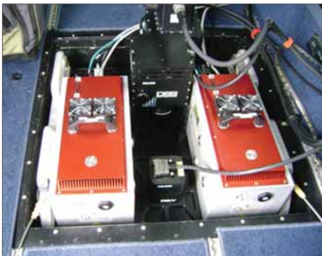
Figure 3-17. The NOAA/NGS’ Riegl LMS-Q690i Dual system (left) and data acquired over the Virginia Coast Reserve in a shoreline test project (right).
