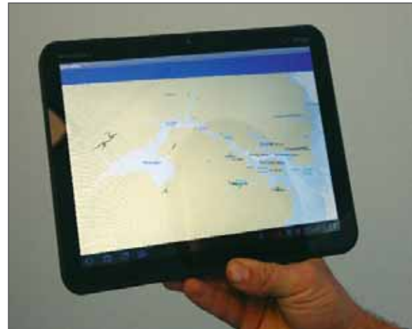
Figure 8-7. Mobile version of the GeoCoastPilot showing some S57 chart data in a view with the orientation controlled by the device's orientation.
