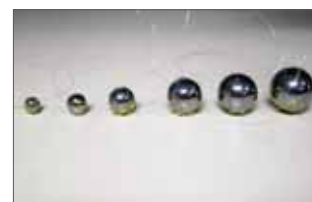
Figure 3-5. Six tungsten-carbide target spheres (10-28 mm) used for measuring combined beam patterns in the near-field.
