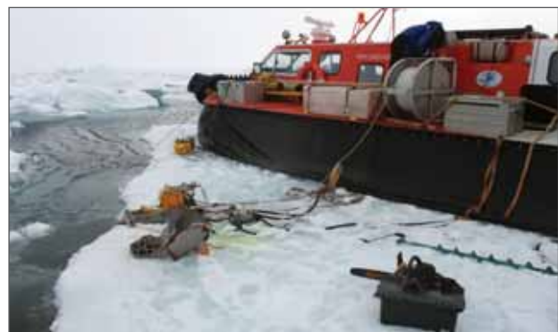
Figure 1-8. Hovercraft dredging operation. The hydraulically powered take-up reel holds lengths of 1000 m of kevlar aramid fiber line with 2 ton breaking strength. All the strain is taken by the hydraulically powered capstan at the ice edge. Note the lightweight dredge with basalt rocks inside. Lines into the water beyond are to an echo-sounder and CHIRP transducers, as well as hydrophones for concurrent air-gun seismic work.
