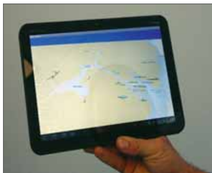
Figure ES-14. Mobile version showing S57 chart data to test viability of using spatially oriented hand-held devices.
