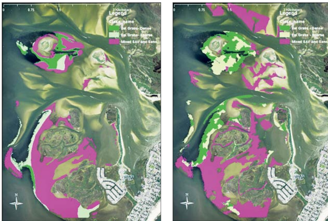
Figure ES-19. Habitat map from Barnegat Inlet generated using manual classification using imagery alone (left) and eCognition classification using lidar and imagery (right).
