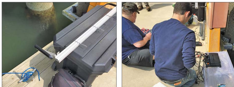
Figure ES-7. Garmin GT-30 sidescan/downscan transducer (left) and GCV-10 black-box sonar module (right), being tested for Trusted Community Bathymetry applications at the UNH pier in New Castle, NH on 2015-06-08.
