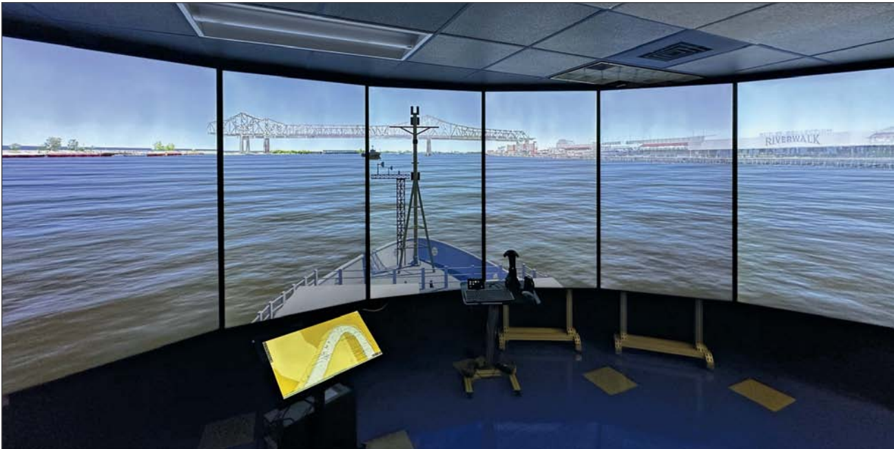
Figure ES-35. The Visualization Lab's semi-immersive tiled display running a head-tracked bridge simulator with accessory monitor that can display ECDIS (reflecting a virtual ship's position/orientation) and augmented camera feeds generated from a virtual camera.
