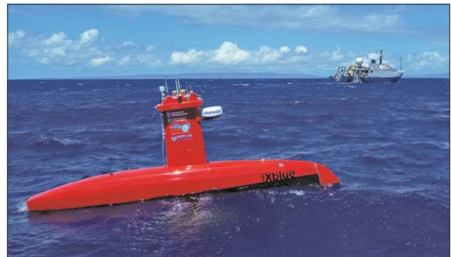
Figure ES-11. DriX was also used to map shallow waters around Nihoa Island while E/V Nautilus mapped in deeper water or in tandem (right).
