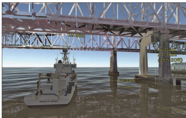
Figure ES-32. Real-time clearance annotations between a 3D model of NOAA's Ronald H. Brown and the Crescent City Connection bridge, based on live data pulled from the PORTS air gap sensor located on the bridge.
