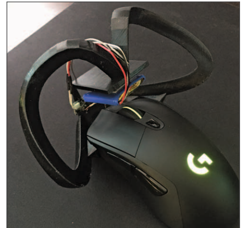
Figure ES-26. Left: Interactive point cloud editor being used on a standard 2D desktop monitor, where the 6DOF handheld controllers can be used to “reach into the screen” and edit, manipulate, reposition, and scale data similar to the immersive mode. Right: Newly developed hybrid mouse/controller that allows interactive editing and full mouse controls with same hand.
