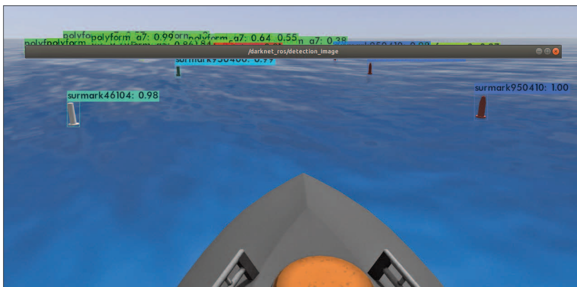
Figure ES-13. Object detections from the ASV's camera during the Virtual Ocean Robotics Challenge.
