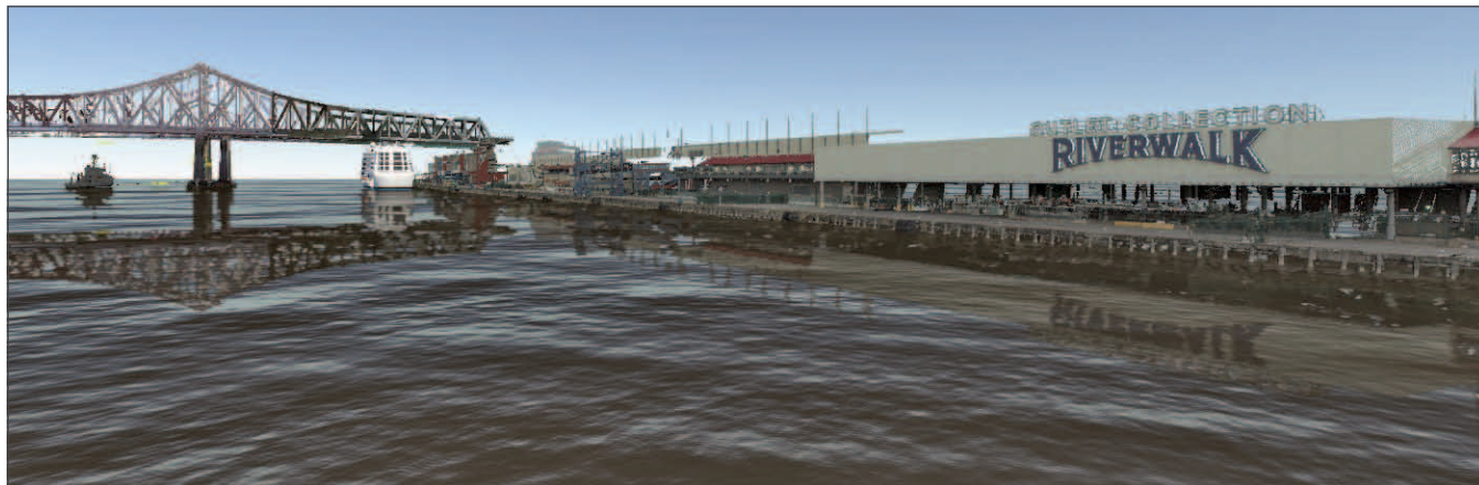
Figure ES-30. A screenshot from the new simulator, showing lidar point clouds of bridges, shorelines, and buildings. Note that features as small as individual boardwalk pilings and ladder rungs are captured.
