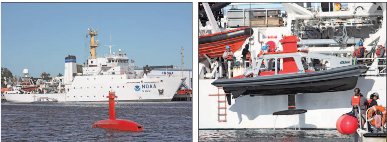
Figure ES-8. Trials of the DriX ASV aboard the NOAA Ship Thomas Jefferson .
