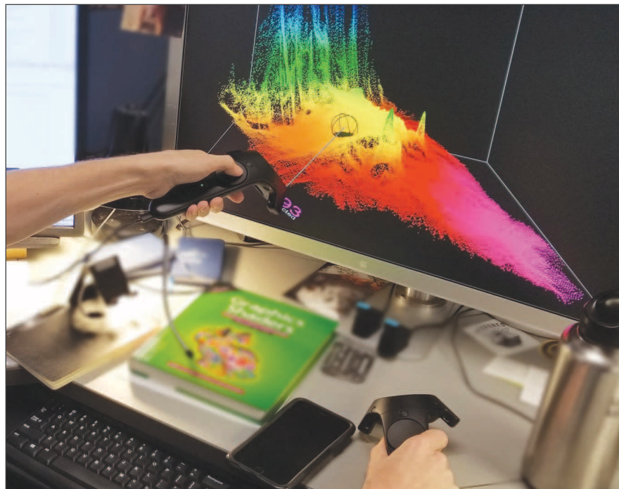
Figure ES-34. Interactive point cloud editor being used on a standard 2D desktop monitor, where the 6DOF handheld controllers can be used to “reach into the screen” and edit, manipulate, reposition, and scale data similar to the immersive mode.
