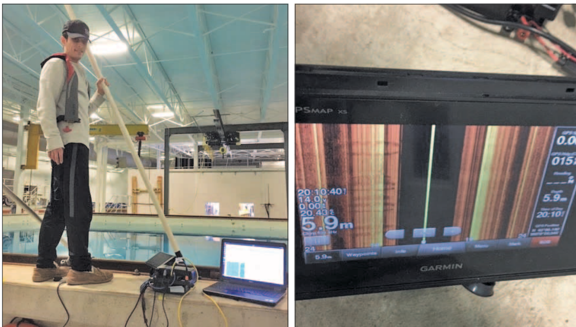
Figure 12-1. Development of a TCB interface for a recreational-class sidescan sonar. In order to determine where particular components of the data appear in the network packets, a sealed (highly acoustically reflective) PVC pipe was used (a) to affect the output of the sonar (b).
