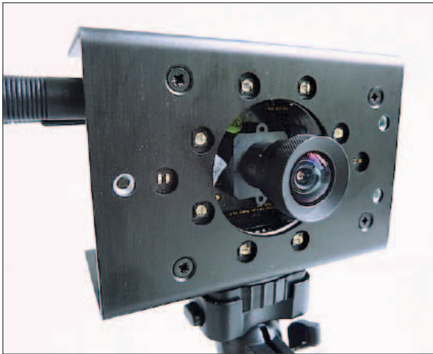
Figure 27-2. ESPROS evaluation kit with IR light sources.
