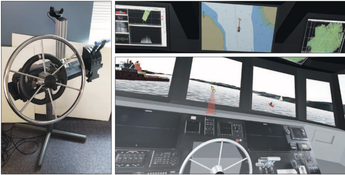
Figure 44-2. The virtual bridge and AR simulator (left). The physical controls used to pilot the boat (below right). View from the virtual bridge within the field-of-view study environment, showing ship traffic and AR trackline to next waypoint (above right). The virtual ECDIS display above the bridge windows, showing a track-up OpenCPN chart with the same trackline and waypoint.
