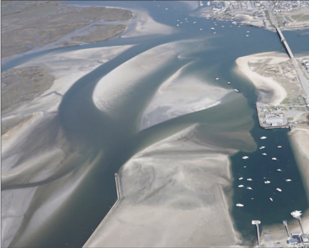
Figure 33-8. Aerial photograph of Hampton/Seabrook Harbor taken in 2017 showing the channel cuts across the middle ground (flood tidal delta) and infilling of the navigational channel leading to a large portion of New Hampshire's fishing fleet.
