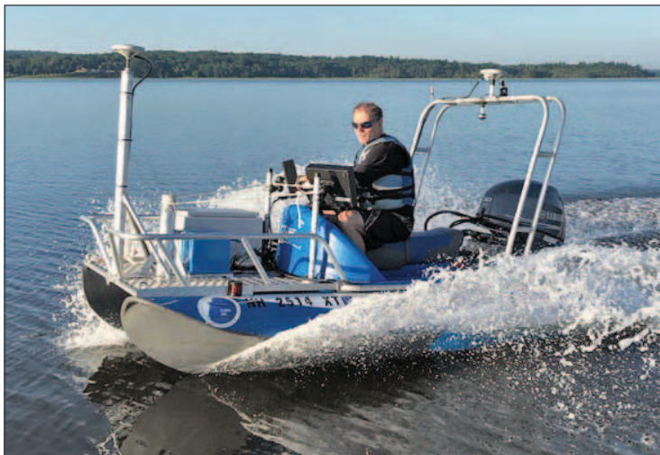
Figure I-14. The JHC Zego Boat, a highly maneuverable and stable twin-hulled catamaran that is being outfitted into a state-of-the-art shallow water survey vessel with MBES, SBES, and ADCP capabilities.
