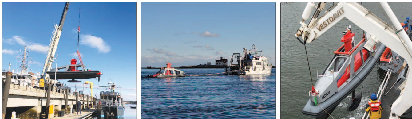
Figure I-18. The iXblue DriX autonomous surface vehicle in its Launch and Recovery System (LARS). From left: being lowered into the water alongside the UNH Marine Pier in New Castle, NH; undergoing testing in Portsmouth Harbor, NH with the R/V Gulf Surveyor; and being launched over the side of the NOAA Ship Thomas Jefferson in Norfolk, VA.
