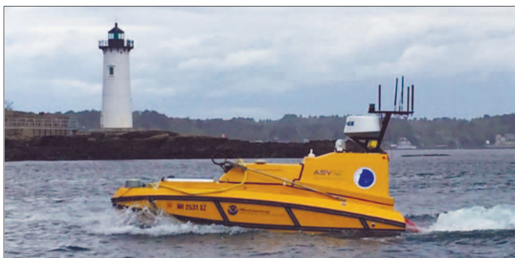
Figure I-16. CWorker-4 model vehicle BEN (Bathymetric Explorer and Navigator) operating in the vicinity of Portsmouth Harbor, NH.
