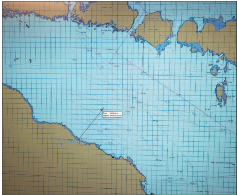
Figure 11-3. ASV-BEN, conducting test of sustainable telemetry range with the Kongsberg Marine Broadband Radio telemetry system. Here the ASV is some 20 km from the operating station, approaching the center of Lake Huron. This range resulted from exceptionally favorable conditions. More typical maximum ranges were 14-16 km.
