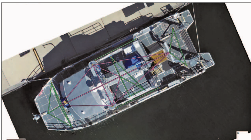
Figure 12-5. Orthomosaic of the R/V Gulf Surveyor corresponding to the point-cloud of Figure 12-3. Note the lines joining survey monuments (purple) and Secchi targets (green), which are measured in the orthomosaic to assess the technique.
