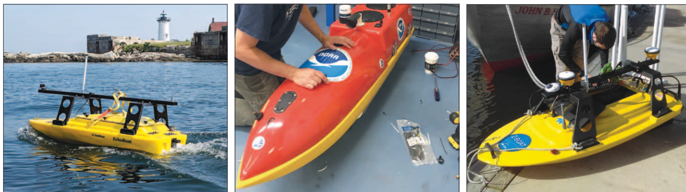
Figure I-17. Small autonomous surface vessels used by the Center to develop autonomous command and control algorithms: Seafloor Systems’ “Echoboat” (left), Hydrnalix “Emily Boat” (middle), and Teledyne Oceansciences’ “Z-Boat” (right).
