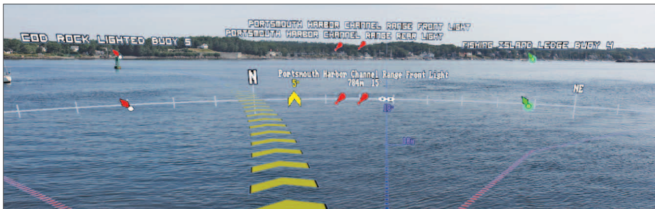
Figure 44-1. Simulated augmented reality overlay of nautical chart information.
