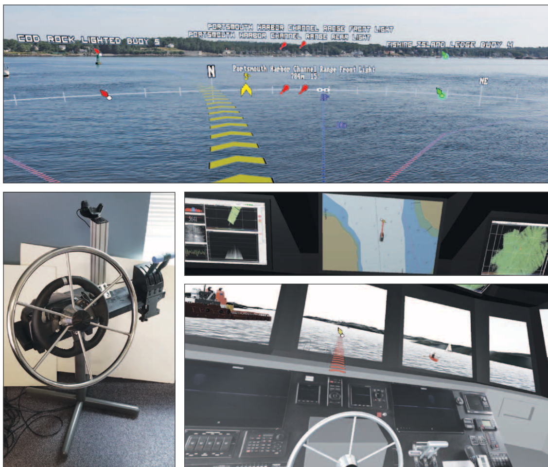
Figure ES-36. Upper: Simulated augmented reality overlay of nautical chart information. Lower: The virtual bridge and AR simulator. Lower Left: The physical controls used to pilot the boat. Above Right: The virtual ECDIS display above the bridge windows, showing a track-up OpenCPN chart with the same trackline and waypoint. Below Right: The view from the virtual bridge within the field-of-view study environment, showing ship traffic and AR trackline to next waypoint.
