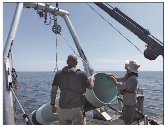
Figure 14-4. The pipe with a 'roughened' surface consisting of antiskid tape and a wrap of potwarp (left image), and the deployment of the pipe at sea using the R/V Gulf Surveyor .
