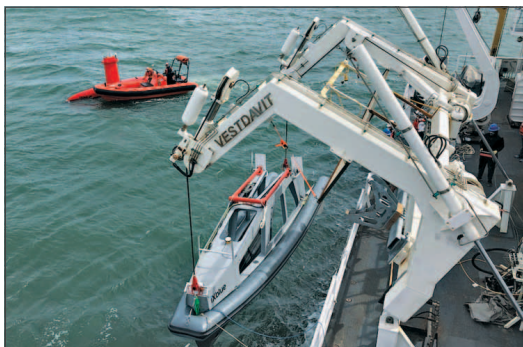
Figure 11-13. Trials of the DriX ASV aboard the NOAA Ship Thomas Jefferson .
