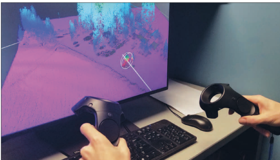
Figure 39-2. Editing coastal LIDAR point clouds with the latest version of our desktop editor, which uses a 3D monitor and 6DOF handheld controllers.
