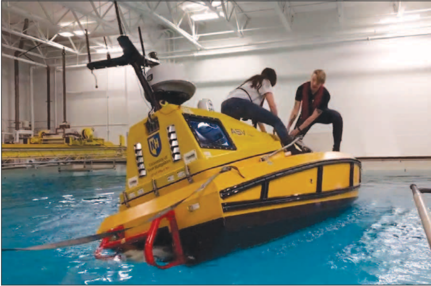
Figure I-7. Engineering test tank being used to test the IMU and multibeam on the BEN (Bathymetric Explorer and Navigator) ASV.
