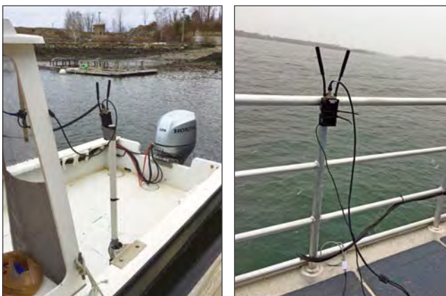
Figure 11-3. Streamcaster Silvus Radio installations for a snowy day of testing aboard the R/V Galen J. (left) and R/V Gulf Surveyor (right).
