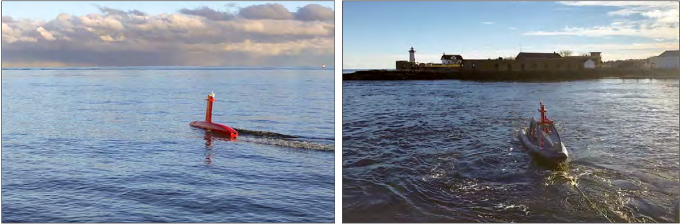
Figure 11-24. The DriX surveying at sea (left) and within the DDS (right).
