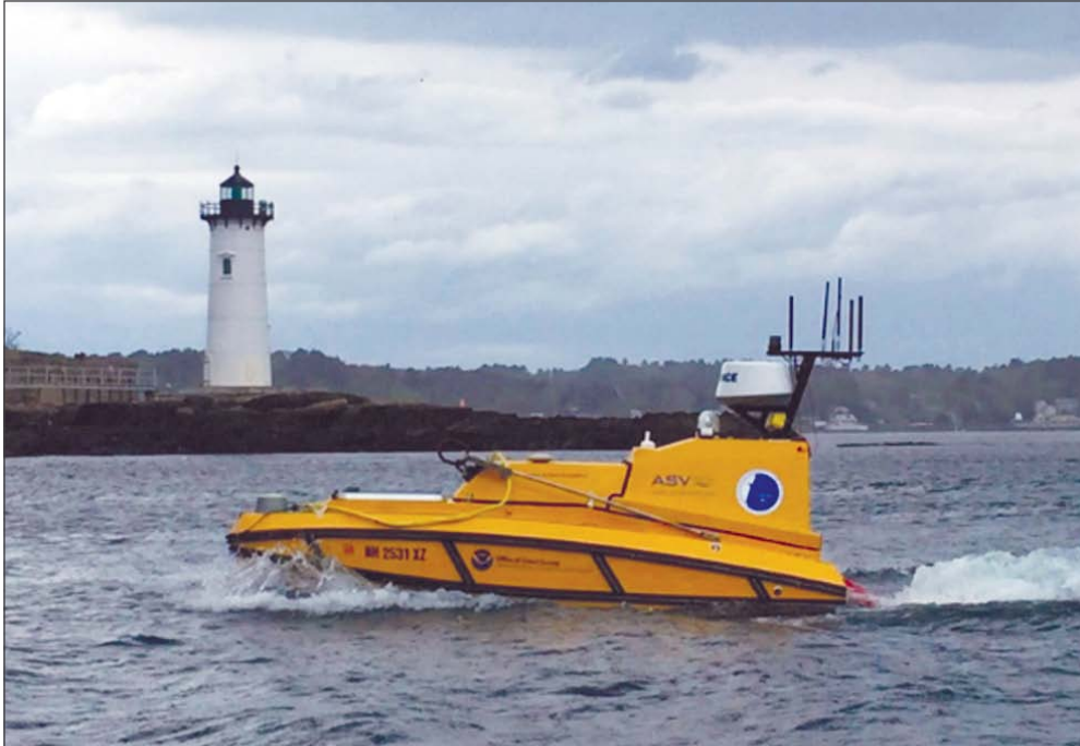
Figure I-15. CWorker-4 model vehicle BEN (Bathymetric Explorer and Navigator) operating in the vicinity of Portsmouth Harbor, NH.
