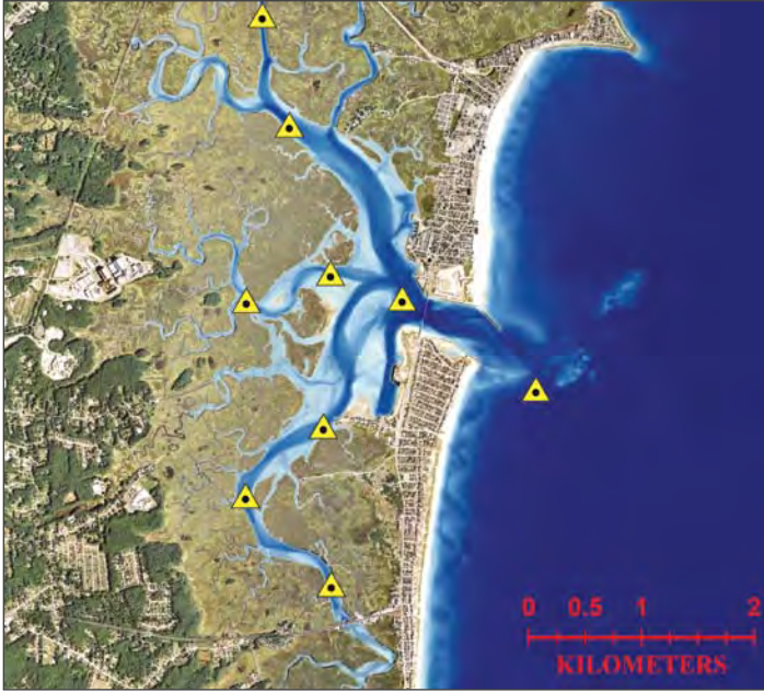
Figure 33-1. Map of Hampton Harbor showing the location of instruments deployed for 30 days in the fall of 2017 to measure wave, currents, temperature, salinity, and optical backscatter. Data from these instruments will be used to verify the hydrodynamic model and set the proper bottom boundary condition for the model.
