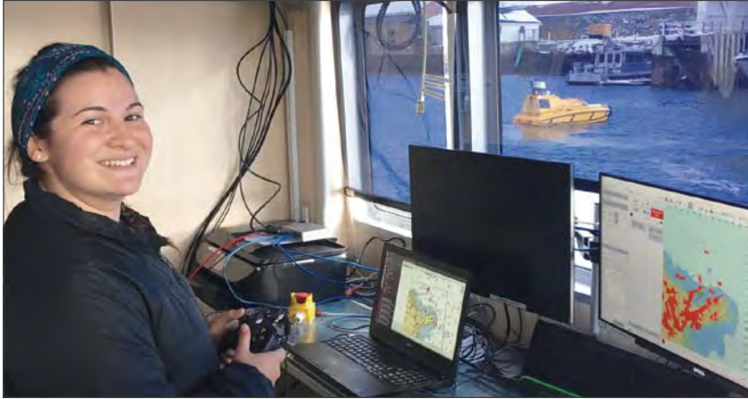
Figure 11-12. Olivia Dube, Ocean Engineering undergraduate, and ASV Group intern, testing an X-box controller for remote piloted operation of the Center's C-Worker 4 ASV.
