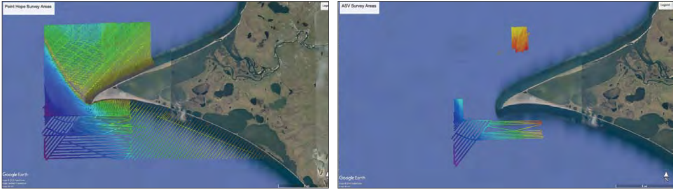
Figure ES-17. The overview image on the left shows combined survey coverage by NOAA and BEN (197 km 2 ) in the vicinity of Point Hope, AK. This overview map includes data collected over 21 survey days by NOAA launches and 6 survey days for BEN. The right image shows BEN's contribution alone (27 km 2 )
