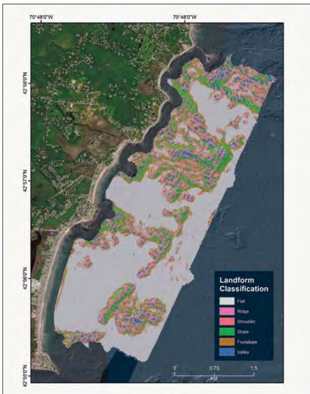
Figure 21-2b. Landforms identified by BRESS analysis applied to the bathymetry shown in Figure 21-2a.
