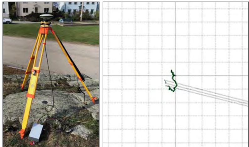
Figure 12-3. Harxon GPS500 antenna being tested for accuracy over an NGS horizontal control mark (AB2631) in New Castle, NH on 2018-05-09. The RTKLib wanderplot for the observations, absent some outliers, shows tight clustering of the solutions as the constellation moves overhead. Scale divisions are 0.01m.
