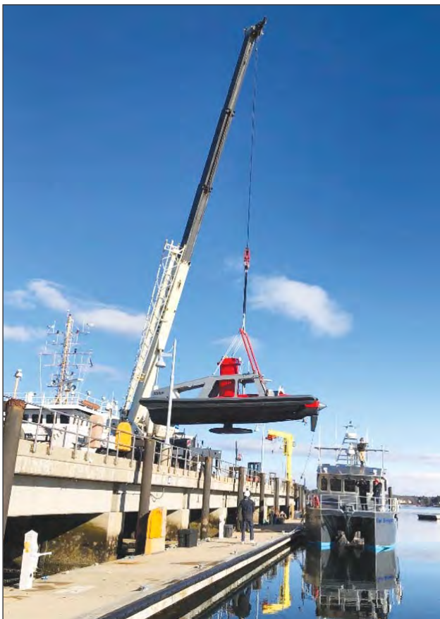
Figure 11-23. Craning the DriX into the water at the UNH Pier.
