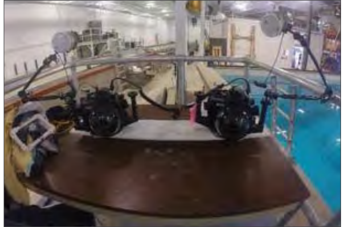
Figure 27-6. Two DSLR cameras are comprising a stereo system on a Delrin board.
