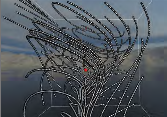
Figure 45-5. Stream tube visualization of a 3D vector field around a critical point (red sphere).
