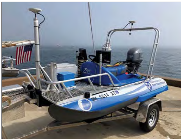
Figure I-14. The JHC Zego Boat, a highly maneuverable and stable twin-hulled catamaran that is outfitted as a state-of-the-art shallow water survey vessel with MBES, SBES, and ADCP capabilities.
