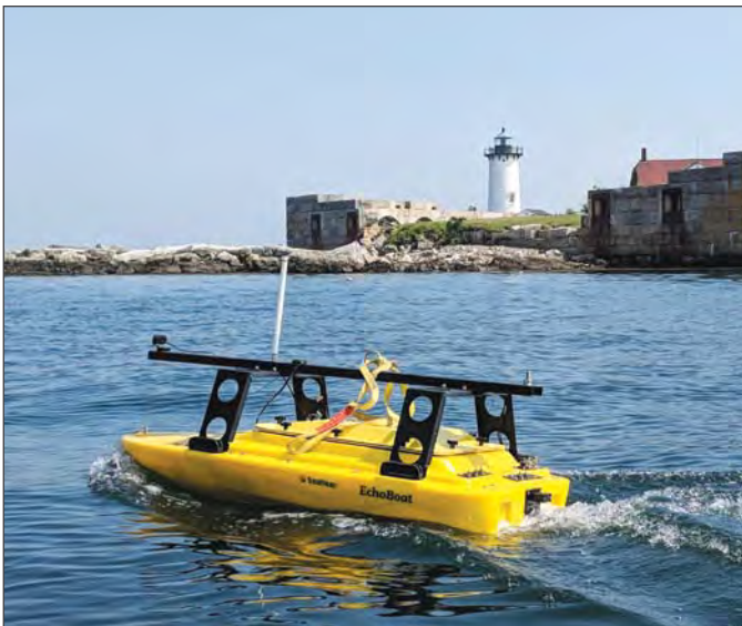
Figure I-16. Seafloor Systems' "Echoboat" (left) and Teledyne Oceansciences' "Z-Boat" (right) — small autonomous surface vessels used by the Center to develop autonomous command and control algorithms.
