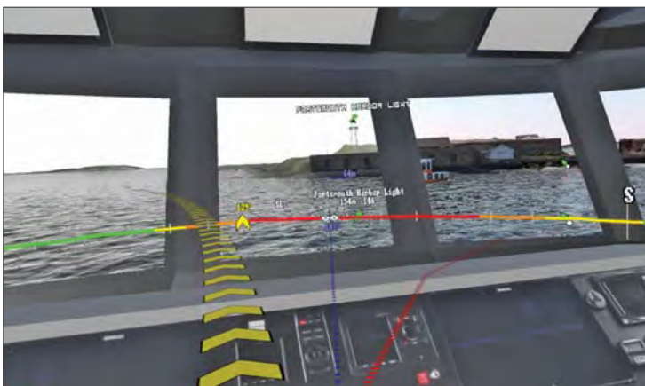
Figure 41-1. Mock-up of the forecast risk applied as a color-code to the compass ring in the virtual reality ship simulator (see Task 44), where red indicates a high risk of continuing in the given direction, and green indicates lower or no additional risk within the forecasting window.
