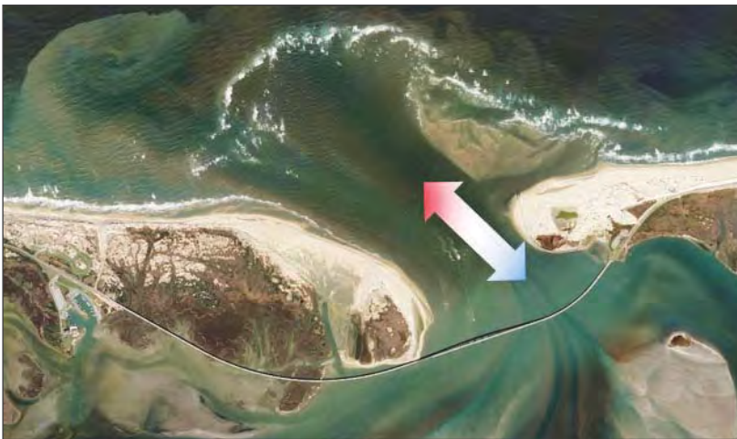
Figure 33-11. Differences in sub-tidal water level variations across the inlet create a dynamic residual pressure gradient which primarily forces a sound to ocean flow.
