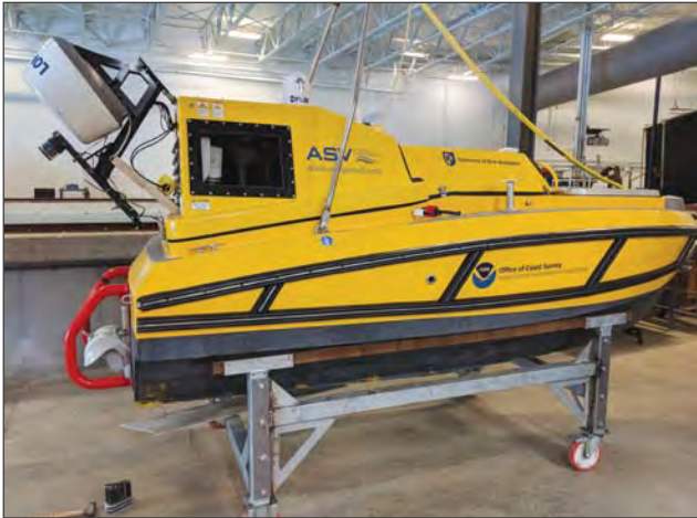
Figure 11-10. Here the ASV’s antenna mast redesign is shown in the rotated back into its shipping position. This modification allows the vessel to be shipped on its trailer in a standard shipping container.
