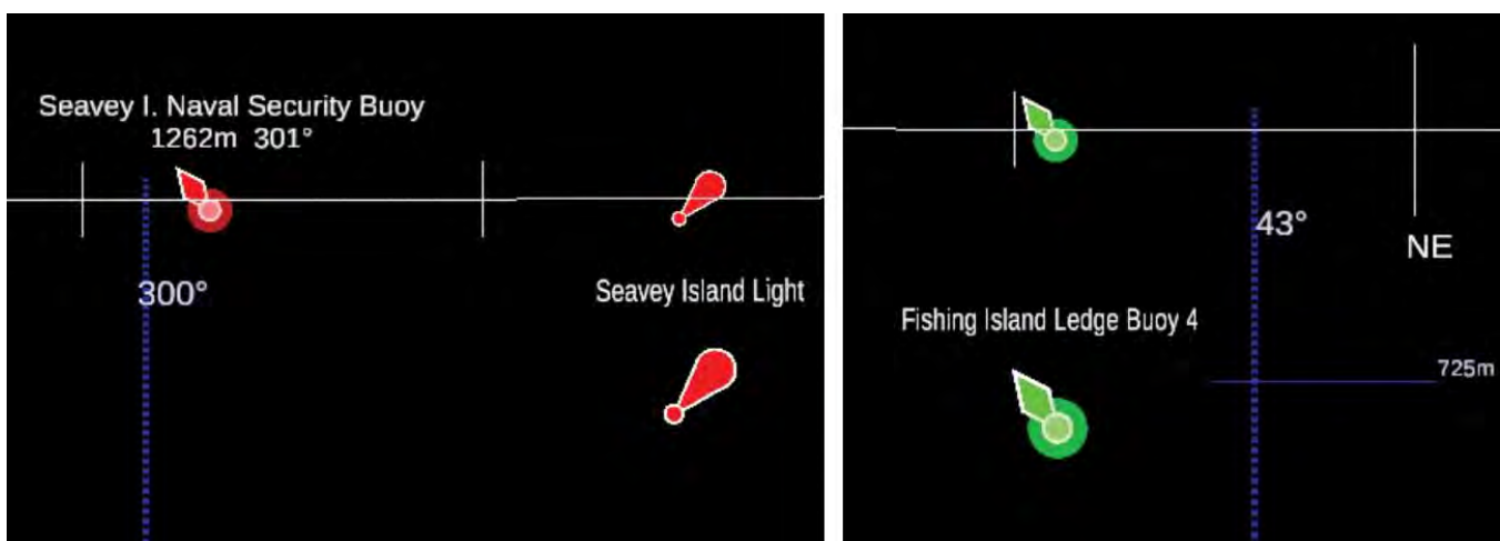
Figure 44-4. Debug views of AR markers, redesigned for maximum brightness and contrast for use on HoloLens. The compass ring was relocated above the horizon to accommodate for HoloLens' restrictive field-of-view.
