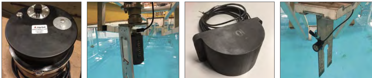
Figure 1-1. Some of the transducers tested in the acoustic tank in 2018. From left to right: EdgeTech DW216; Imagenex DeltaT; Prototype projector from EdgeTech; Hydrophone from Mitre Corporation.
