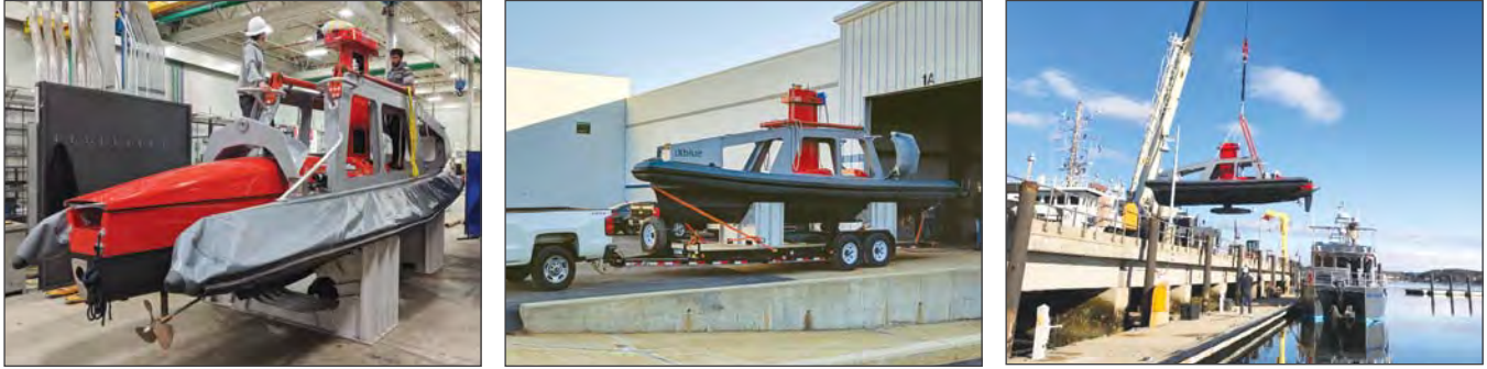
Figure I-17. iXblue DriX autonomous surface vehicle in its Launch and Recovery System (LARS) (l-r) arriving at the facility where it will be evaluated, trailed for transport to the UNH Marine Pier in New Castle, NH, and being lowered into the water alongside the pier.
