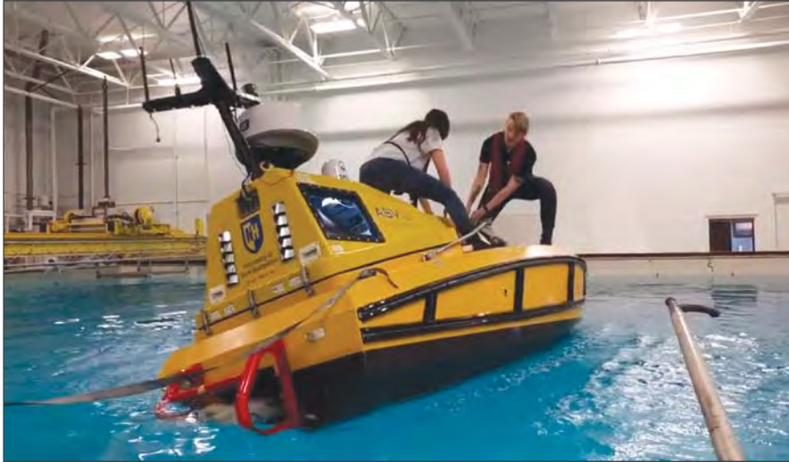
Figure I-6. Engineering test tank being used to test the IMU and multibeam on the BEN (Bathymetric Explorer and Navigator) ASV.
