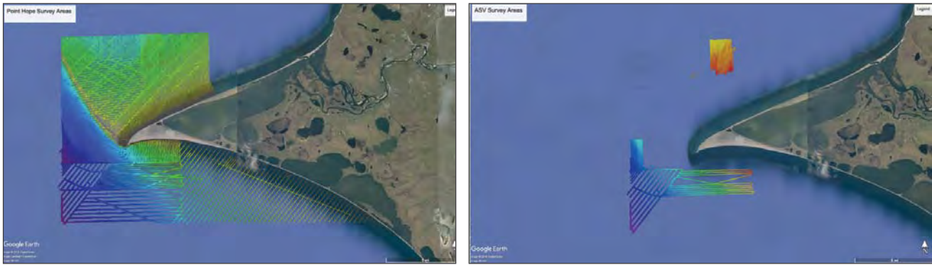
Figure 11-20. The overview image on the left shows combined survey coverage by NOAA and BEN (197 km 2 ) in the vicinity of Point Hope, AK. This overview map includes data collected over 21 survey days by NOAA launches and six survey days for BEN. The right image shows BEN's contribution alone (27 km 2 ).
