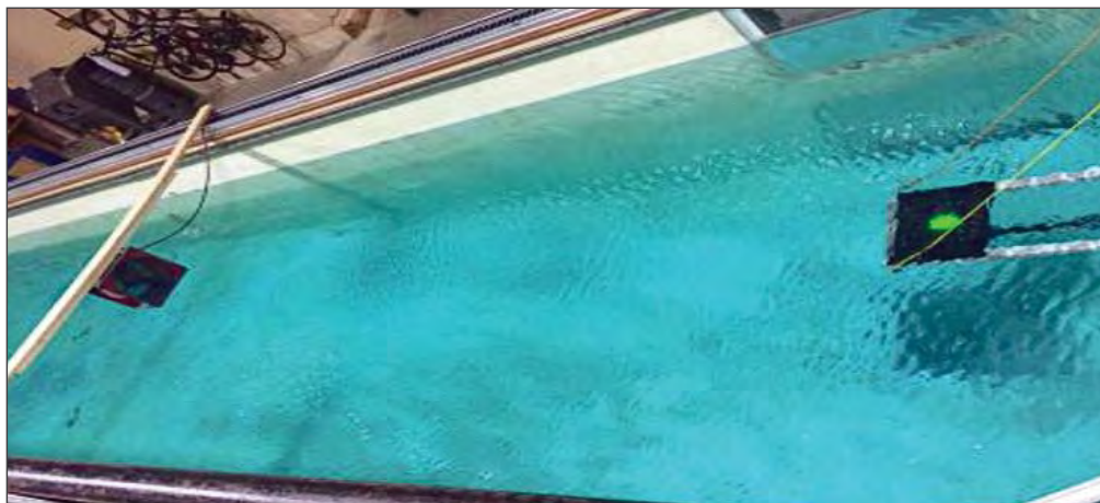
Figure ES-4. Experimental setup at the UNH's Chase Ocean Engineering Lab with the optical detector array and the industrial fan that generated capillary waves.
