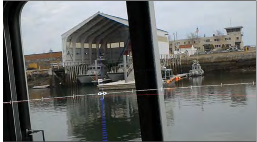
Figure 44-3. Video capture from testing the AR navigation software on a Microsoft HoloLens aboard the R/V Gulf Surveyor .
