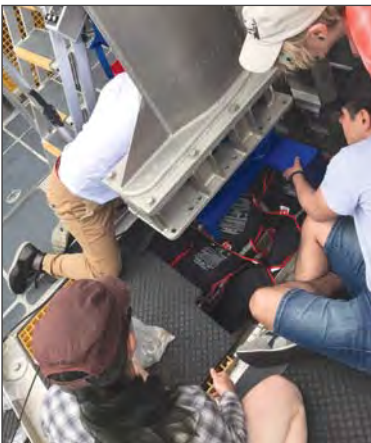
Figure 53-2. Students installing an R2Sonic 2024 multibeam sonar during the mobilization stage of the hydrographic surveying field course.
