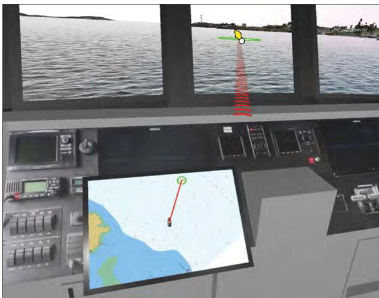
Figure 44-2. AR simulator running the FoV study. Participants can use either the ECDIS screen (lower left) or the FoV AR overlays (over the water) to help them navigate along red track lines to buoys (yellow marker w/ green ring). The system records how often users look down at the display to understand when, for how long, and why users take their eyes off the water.
