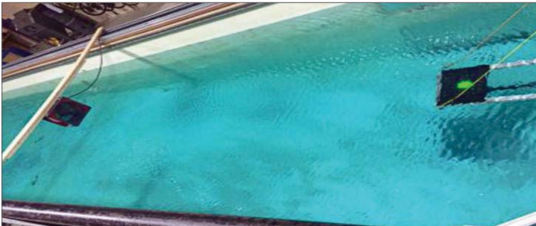
Figure ES-4. Experimental setup at the UNH's Chase Ocean Engineering Lab with the optical detector array and the industrial fan that generated capillary waves.
