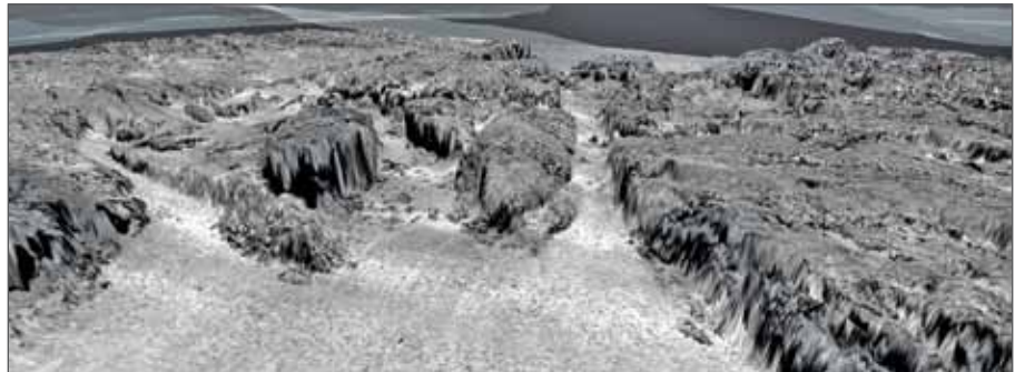
Figure ES-14. Bathymetry draped with acoustic backscatter from the ASV's Kongsberg EM2040p sonar system. This image is shown with no vertical exaggeration.
