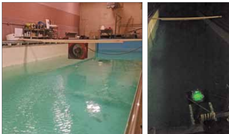
Figure ES-6. Water surface experimental setup. Left: Fan mounted on the tow tank creates capillary surface waves. Right: The optical detector array submerged underwater with the laser beam footprint. The incoming waves change the laser beam footprint location on the array.
