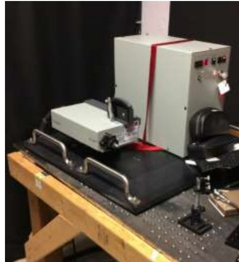
Figure 3-21 (Left) The green pulsed Nd:YAG laser unit (Continuum Minilite) used in the bottom return experiments with mirror guides used for alignment. Right - Materials that were used in the bottom return calculations. (a) white board (b) concrete (c) sand (d) wood
