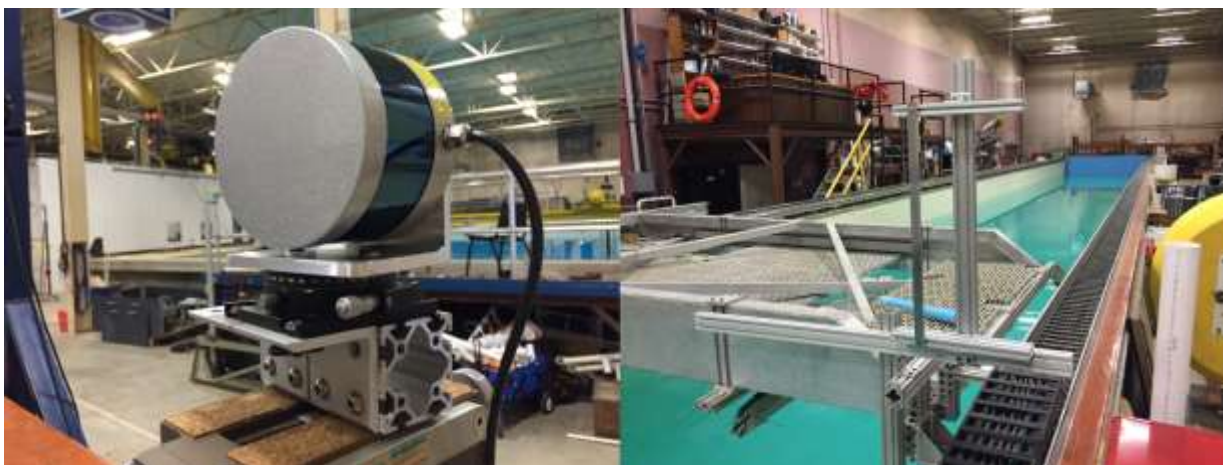
Figure 3-11: Left: Laser scanner mounted vertically centered over the ultra-high precision rotating compass. Right: Narrow vertical aluminum target.
