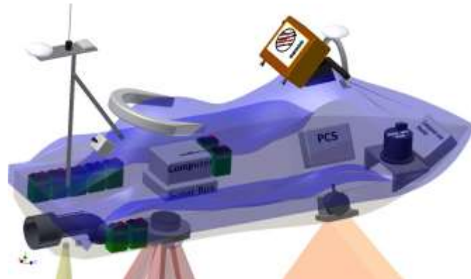
Figure 1-11. CBASS in action surveying in New River Inlet NC (left) and CAD drawing (right) showing the location of the MBES (peach), SBES (yellow), ADCP (red) with acoustic beam patterns on the CBASS. Also shown are the location of the POS MV IMU and PCS, onboard computers and LAN router, internal battery packs, GPS and RTK antennae, and navigational display monitor
