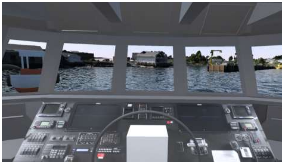
Figure 44-6: Screenshot from within simulator, showing view from inside virtual Gulf Surveyor bridge, with photo-textured instrument panel, looking towards UNH's Newcastle Pier.
