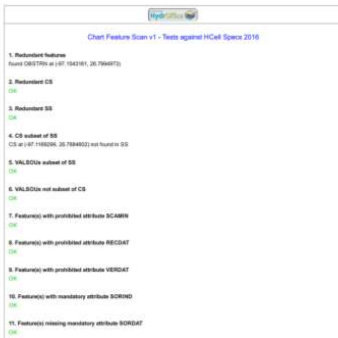
Figure 15-13: Feature Scan of prospective chart components quickly catches a multitude of potential minor errors that frequently occur. The PDF summary shown above serves as a useful record for review.
