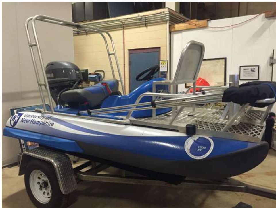
Figure 1-12: The JHC Zego Boat, a highly maneuverable and stable twin-hulled catamaran that will be outfitted into a state-of-the-art shallow water survey vessel with MBES, SBES, and ADCP capabilities.
