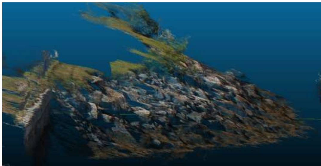
Figure 44-12: Detailed side view of the color point cloud shown in the previous figure, showing the 3D detail of the point cloud capturing the rocks / rip-rap.
