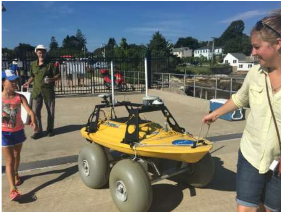
Figure 11-4: The Teledyne Oceansciences "Z-boat" fitted to a wheeled cart typically used for jet-ski deployment from beaches. The cart was found to make for easy transport around the lab and from the Center's truck to various small boats used for deployment.
