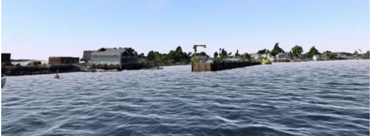
Figure 44-13: Panoramic screenshot from inside the AR simulator showing the models generated through the SfM process using this 394 photo dataset.
