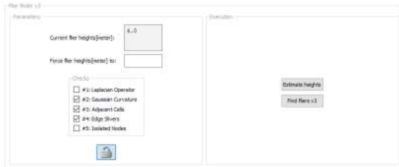
Figure 15-4: Flier Finder 3 offers an automated estimation of search height, to increase standardization of the tool for RSA purposes, though a custom height may be forced. The various algorithms to detect anomalous grid data may be enabled or disabled as desired, but the default algorithms of Gaussian Curvature and Adjacent Cells were built to minimize false positive detections, while Edge Slivers focuses on grid edges where anomalous data is routinely observed. Laplacian Operator may be used as needed for a finer search, and Isolated Nodes with search for grid data far detached from the grid and perhaps unintentionally retained.
