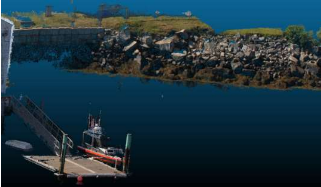
Figure 44-11: Color point cloud of the waterline/shoreline at Fort Constitution and New Castle Coast Guard station.
