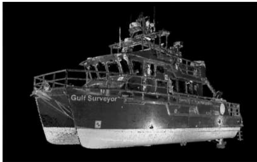
Figure 1-8: Laser Scan point cloud of R/V Gulf Surveyor
