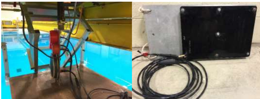
Figure 1-2. Some of the transducers tested in the acoustic tank in 2016. Left: Simrad ES120 and 200 and MSI Constant Beamwidth Transducer; Right: Edgetech PVDF transducer.
