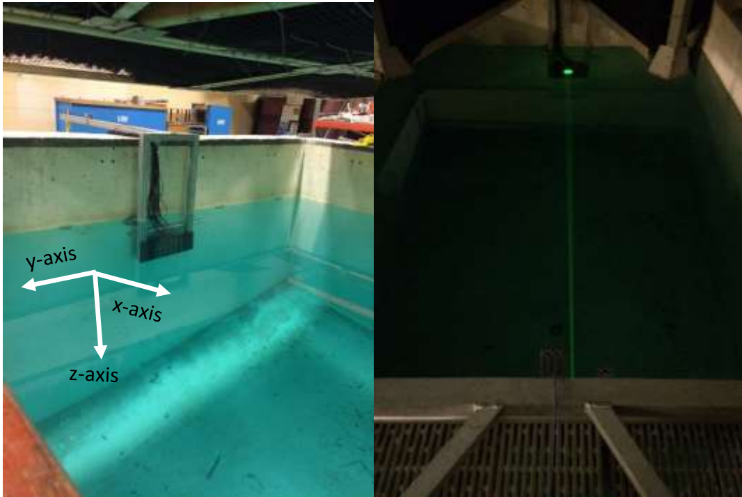
Figure 5-3: Left: Optical detector array mounted vertically for water column experiments. Right: laser beam ray-path geometry in the water column. The detector array intersects the laser beam at a specified distance.
