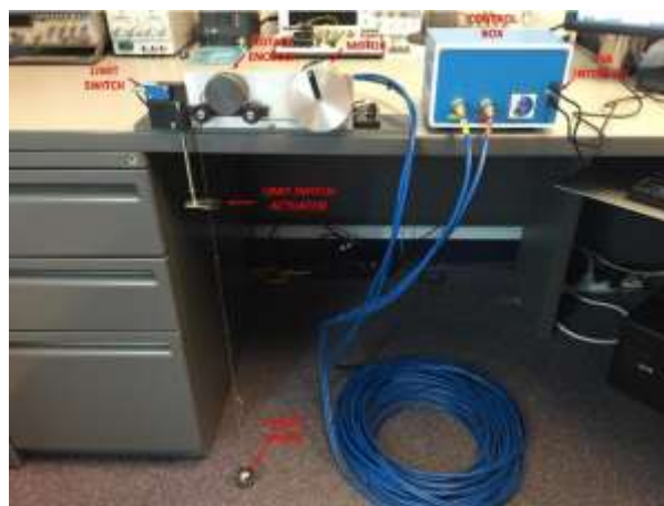
Figure 1.1. Upgraded vertical target positioning system on bench
