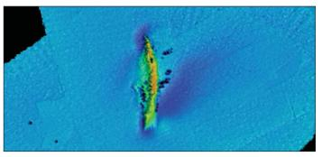
Figure 18. Shipwreck of the Andrea Doria mapped in October 2009 by the NOAA FRV HENRY BIGELOW with the Simrad ME70 multibeam sonar. Data were collected using a standard water column (non-bathymetric) mode.
