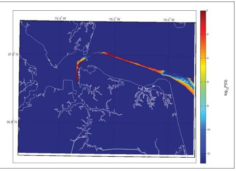
Figure 8. Log. of maximum probability of grounding in each 100 m X 100 m area in the approaches to the Port of Norfolk, based on activity and sizes of the Cargo-class ships associated with the container terminal zone shown in Figure 5. The probabilities are mostly depth related (since these vessels are typically draught-constrained in this area), but some variations due to speed are also observed in the approaches area.
