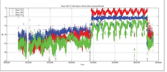
Figure 10. Time series plot of three beams (108, 110, 112) showing seafloor and sphere beam averaged backscatter. A 14 inch stainless steel sphere (filled with distilled water) was placed on the seafloor on 05/27/08 and removed on 06/02/08.
