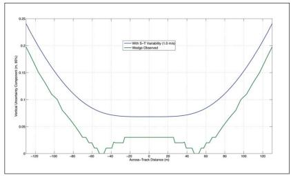
Figure 9. A comparison of the vertical component of uncertainty due to the sound speed spatio-temporal uncertainty using the current model (blue) and an uncertainty wedge analysis (green). The step-effects in the UWA result are due to sampling issues in the wedge construction.
