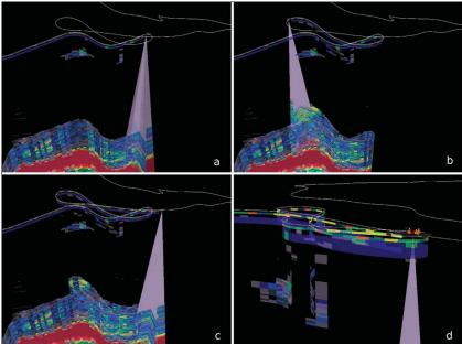
Figure 11. Sequence of passes over a small target near the surface. The real time geo-referenced display of the Simrad EK60 echo sounder data in GeoZui4D was used to steer the subsequent passes over a moving then disappearing target.
