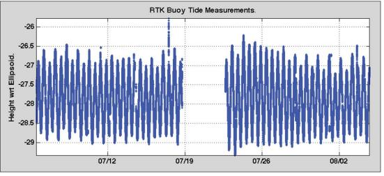
Figure 51: Tide measurements (re: ellipsoidal height) made from RTK-equipped tracking buoy.
