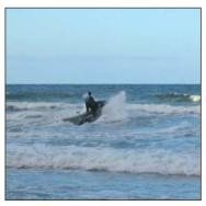
Figure EX-4. CBASS surveying very shallow water through surf.
