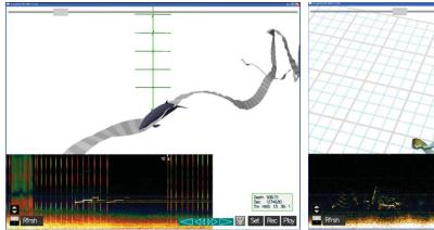
The TrackPlot trajectory of a Cuvier's beaked whale. The plot shows whale clicks and the acoustic signal of a sub-bottom profiler recorded. Both signals recorded from a hydrophone attached to a whale.
