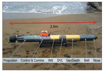
Figure EX-10. GAVIA AUV with GeoSwath Phase Measuring Bathymetric Sonar.
