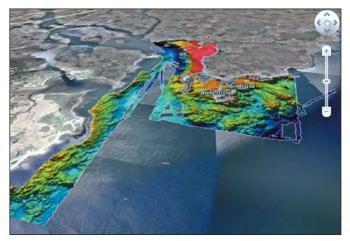
Figure 53. Oblique image showing the bathymetry measured with the CBASS around Portsmouth Inlet overlaid on satellite imagery from Google Earth. The depths range from 0.5-25 m.
