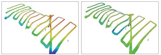
Figure 42. Bathymetry derived from the ME70 data during one of the large scale surveys (red is shallow, blue is deep) is shown on the left. Seafloor backscatter, also derived from the ME70 data (red/yellow indicates higher backscatter, blue indicates lower backscatter) is shown on the right.
