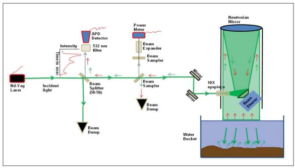
Figure 23. Schematic illustration of the bathymetric LIDAR simulator.
