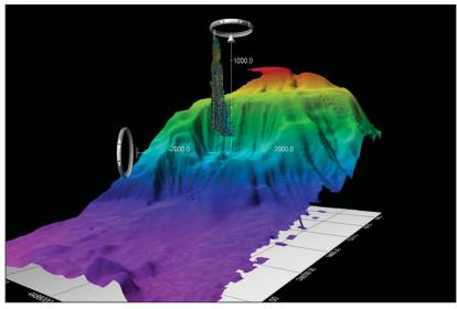
Figure EX-1. 1400 m high gas plume discovered on the Mendocino Fracture Zone by mid-water multibeam sonar on the NOAA Vessel OKEANOS EXPLORER during the initial testing of the multibeam sonar.
