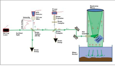
Figure EX-3. Schematic illustration of the bathymetric LIDAR simulator.
