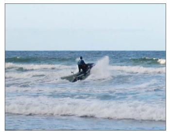
Figure 52. The Coastal Bathymetry Survey System (CBASS) operating in an energetic surf zone. The CBASS is equipped with single-beam echo-sounder and differential GPS, and is capable of measuring the bathymetry in shallow water with accuracies on the order of 0.10 m.
