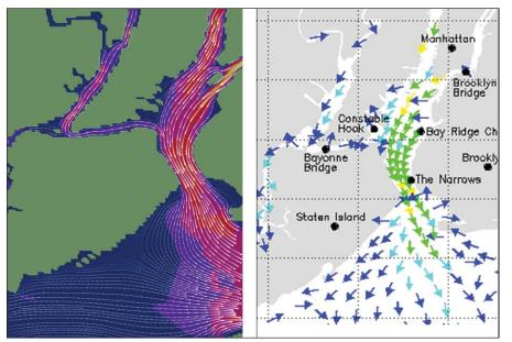
Figure 14. FlowVis2D representation in NowCOAST of the New York Operational Forecast System (left)—contrast this with the standard representation (right).
