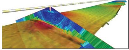
Figure EX-8. ME70 water column and seafloor bathymetry visualized in the new Fledermaus mid-water tool (bathymetry processed off-line by CCOM/JHC software).
