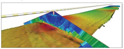
Figure 41. ME70 water column and seafloor bathymetry visualized in the new Fledermaus midwater tool (bathymetry processed off-line by JHC/CCOM software).
