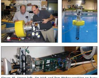
Figure 49. Upper left: Jim Irish and Tom Weber working on buoy #1 in the lab. Upper right: buoy #1 floating in the acoustic test tank during initial testing. Bottom: the 'guts' of buoy #1.
