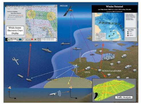
Figure 33. AIS binary message broadcast scheme for Right Whale locations in Stellwagen Bank National Marine Sanctuary.
