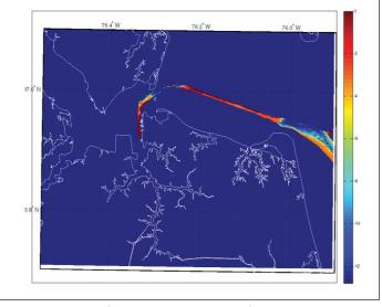
Figure EX-2. Log. of maximum probability of grounding in each 100 m x 100 m area in the approaches to the Port of Norfolk, based on activity and sizes of the Cargo-class ships associated with the container terminal.
