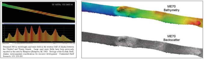
Figure 17. Bathymetry and backscatter in the Shumagins (western Gulf of Alaska) showing rock outcroppings. Depths range from 80-120 m over the 6 km long transect. Data were collected using the ME70 multibeam echo-sounder, processed in custom MATLAB software, gridded and then plotted in Fledermaus. Note that the raw soundings processed in MATLAB have not been cleaned, giving an indication of the fidelity of the ME70 data.
