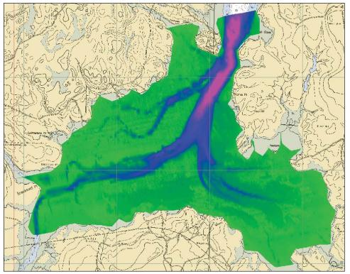
Figure 54. Results of the 2009 Great Bay survey. Note that the presence of eelgrass can be observed by an increased noise level. This data has great potential for post processing with the TracEd tool.
