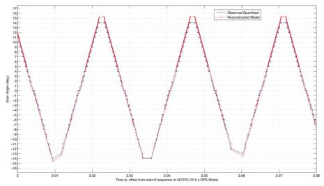
Figure 20. Example of observed, quantized, topographic LIDAR scan angles and reconstructed model angles using a Bayesian estimator. Effects of pattern irregularities, which appear to be active roll-stabilization of the LIDAR, cause complexities in the estimation that are not readily resolved using simpler estimators.
