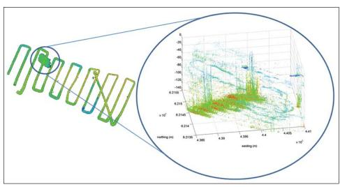
Figure EX-9. Seafloor backscatter from (a proxy for bottom type), and the water column backscatter (Sv) from the highlighted area collected with ME70 on DYSON. In the highlight, apparent bubble plumes appear light blue with a high vertical extent and narrow cross section. Rockfish appear aggregated in a 'carpet' around the base of the plumes (red and green.
