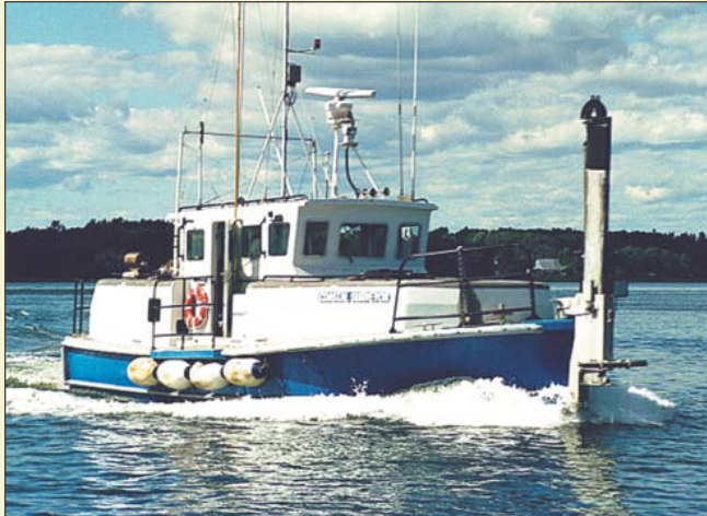
Figure 3. R/V Coastal Surveyor with bow ram.
