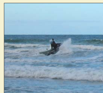
Figure 31. The Coastal Bathymetry Survey System (CBASS) operating in an energetic surf zone. The CBASS is equipped with single-beam echosounder and differential GPS, and is capable of measuring the bathymetry in shallow water with accuracies on the order of 0.10 m.
