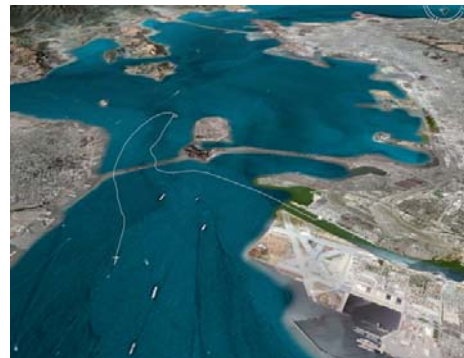
Path of containership Cosco-Buson monitored through AIS at CCOM/JHC soon after collision with the San Francisco Bay Bridge
