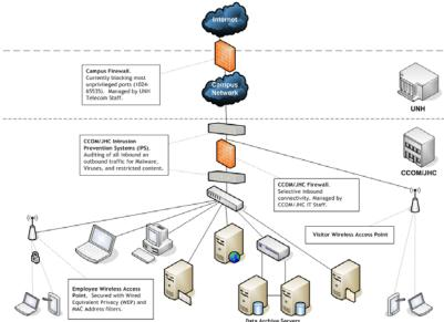
Fig. 2. Current topology of JHC computer network
