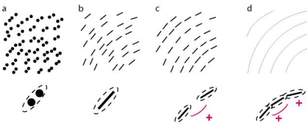
4. TOP: a set of methods which have been used for flow visualization. Note that there are no arrowheads here and so the direction of flow is ambiguous. BOTTOM: the predicted effect of the patterns generated by each method on orientation selective neurons.
