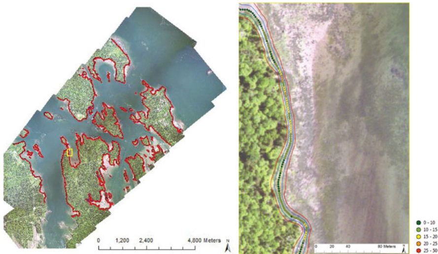
Figure 9. The uncertainty boundaries. The blue lines and the red lines represent the standard uncertainty and the uncertainty at the 95% confidence level, respectively. The black lines are the MHW shoreline. (Left) the imagery for the whole study area. (Right) the enlarged imagery for the yellow box in the left imagery. The points with different colors represent the slope in degree.
