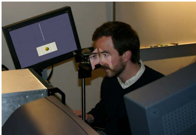
Figure 4. The Wheatstone stereoscope display. The image on the screen has been added using Photoshop.
