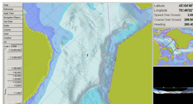
Figure 5: A sample configuration of the GeoNav3D interface. At center is a view of the immediate surroundings of the vessel, while at right are a map overview and a cutaway view from behind the vessel (good for illustrating lateral tolerances in a channel).
