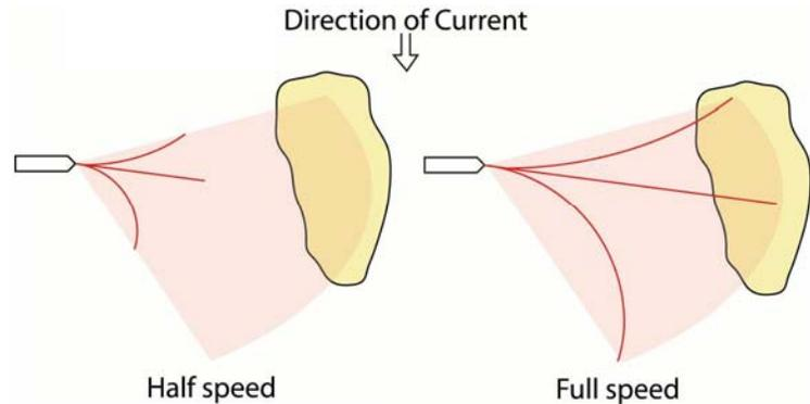
**Figure 3:** An illustration of how vessel modeling could aid a mariner in determining where a vessel will be at given rudder angles and engine speeds, while accounting for the depth of the water underkeel.
