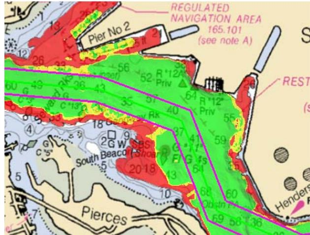
**Figure 7:** A planned path (bold corridor), along which water levels expected at the time of transit are shown. Outside the corridor, water levels are shown for the current instant in time (notice the sharp discontinuities along the corridor near Pier No. 2).
