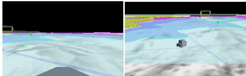
**Figure 4:** 3D views in the reference frame of a vessel. At left is a view from the bridge, while at right is a view from above and behind. Both views can be helpful in aligning what is seen out the bridge window with what is on the computer display.
