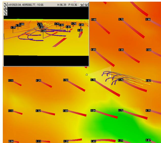
**Figure 6:** A vector field showing currents in the Chesapeake Bay [3] at an instant in time, where each vector is labeled with a magnitude at its origin. Streaks in this vector field illustrate how particles on the surface move, with the dark end representing history, and the light end indicating the current location of such particles.
