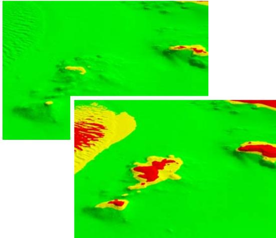
**Figure 2:** Depth areas color-coded based on vessel draft, with green and red colors indicating go/no-go areas. The top frame corresponds to a high water condition while the bottom frame is near MLLW.
