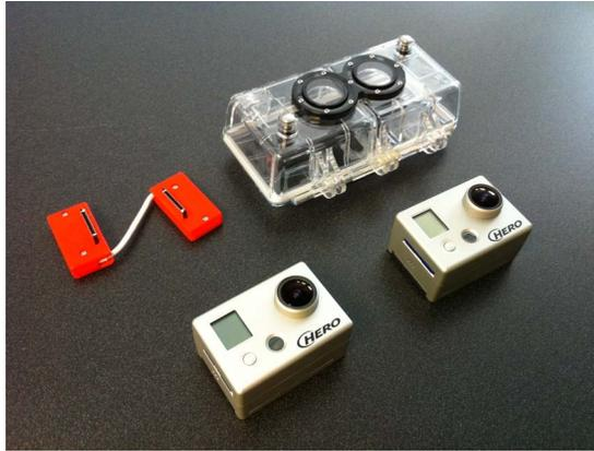
Fig. 1. GOPRO Cameras with stereo housing and synchronization cable.
