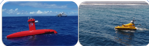
“DriX-8” (DriX vehicle manufactured by iXblue) and “ASV-BEN” (C-Worker 4 vehicle manufactured by ASV Global/L3Harris), are two robotic vessels operated by the Center for hydrographic survey missions.
