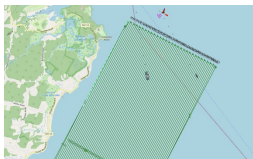
A typical “Boustrophedon” type survey plan run by human and robotic systems for hydrographic survey. Malfunctions and interfering traffic often leave irregularly spaced gaps in the survey, that must be efficiently covered in subsequent work.
