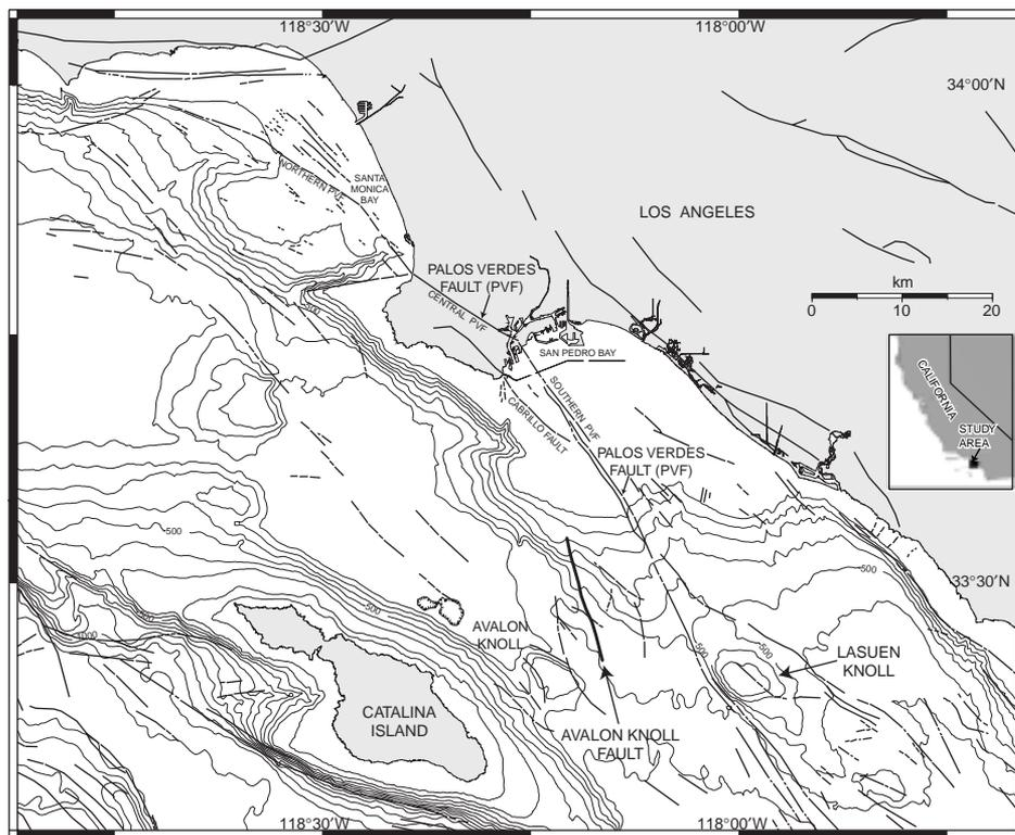
**Figure 1.** Bathymetry and major onshore (Jennings, 1994) and offshore (Greene and Kennedy, 1987) faults of central southern California. Avalon Knoll fault (heavy line) is from this study. Bathymetry is from Smith and Sandwell (1997).
