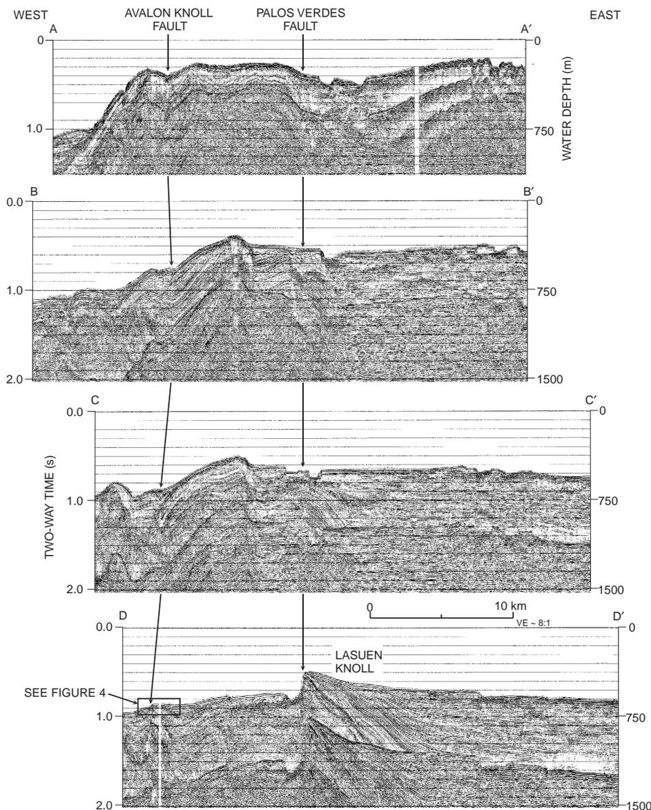
**Figure 3.** High-resolution, multichannel seismic-reflection profiles across continental slope south of San Pedro Bay. Profiles are aligned along trace of Palos Verdes fault. See Figure 2 for profile locations.
