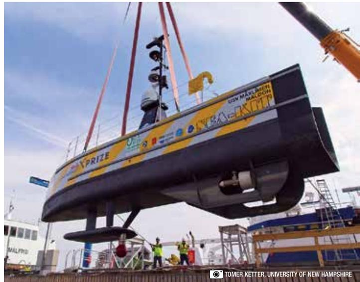
Figure 1: XPRIZE entry SEA-KIT USV *Maxlimer* being deployed for sea trials in Horten, Norway. The sensor gondola below SEA-KIT USV *Maxlimer* contains a HiPAP acoustic navigation system and EM304 multibeam echo sounder system.
