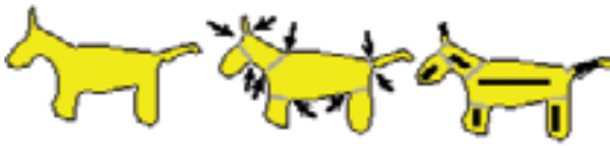
1 According to Marr and Nishihara, 9 concave sections of the silhouette define the object's subparts. These points are critical in defining a structural skeleton. (Adapted from Marr and Nishihara. 9 )
