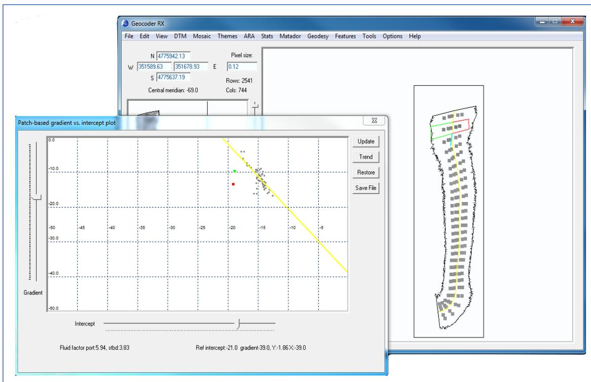
*Figure 2 – Bivariate plot of acoustic backscatter-derived features computed from a half-swath patch of MBES data. The red/green indicated half-swaths have distinctly different behavior (as measured by the slope and intercept of a line fitted to the acoustic backscatter angular response in the patches) from the other patches, an indication of anomalous behavior. Use of multivariate combinations of features can help to clarify detections and reduce false alarm rates.*
