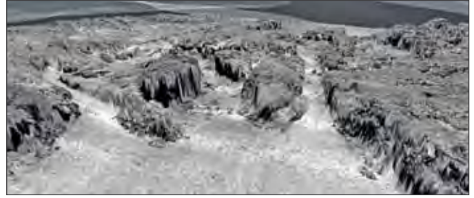
Figure 11-17. Bathymetry draped with acoustic backscatter from the ASV's Kongsberg EM2040p sonar system. This rock outcropping in the vicinity of Santa Barbara Island is shown with no vertical exaggeration.
