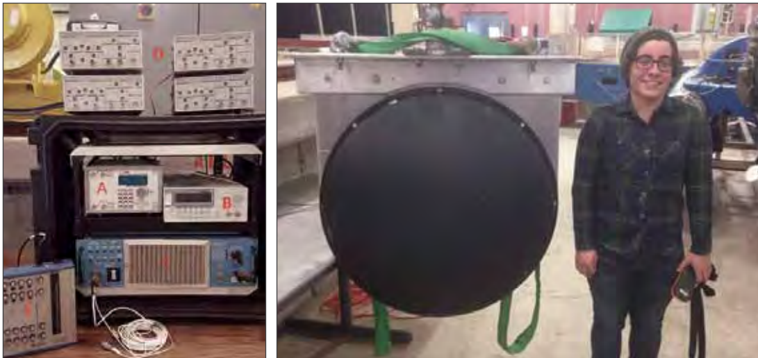
Figure 20-5. Electronic setup to transmit and receive acoustic signal with the Low Frequency Constant Beam Width (LFCBW) transducer. A) Pulse/Delay Generator. B) Arbitrary Waveform Generator. C) Power Amplifier. D) Pre-Amplifiers. E) Data Acquisition Board. Right: LFCBW split-beam echosounder. During this experiment the LFCBW transmitted 10-45 kHz linear-frequency modulated pulse with 2.1 ms pulse length.
