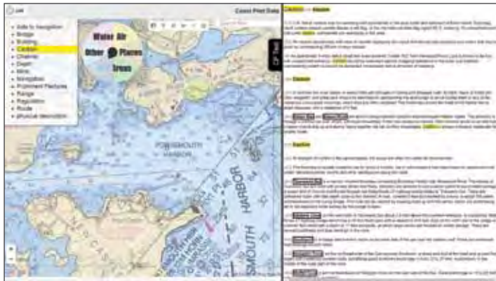
Figure ES-35. Menu selection on Nav yields a list of navigationally significant topics. The CP Text tab is then populated with information related to Cautions in the area for the "Caution" selection.
