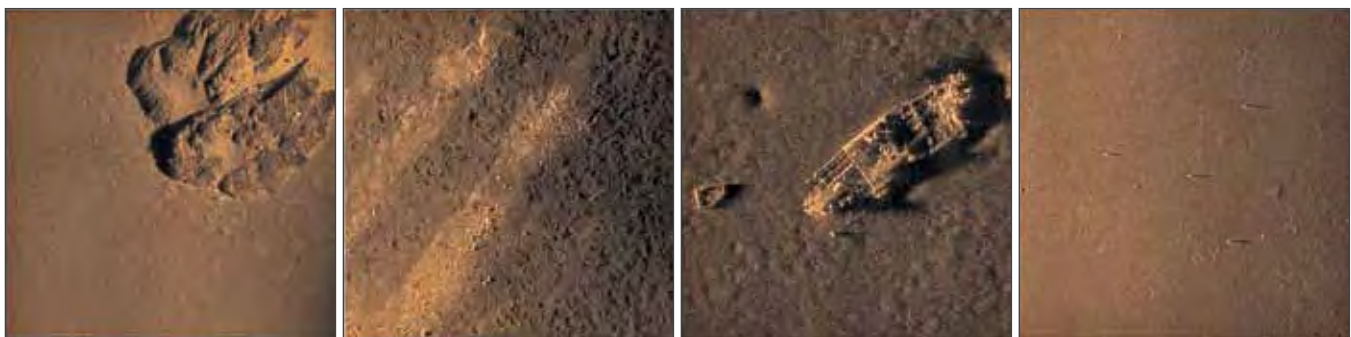
Figure 53-12. Kongsberg Maritime Reflection software spot focus HISAS images (4cm resolution) of geological features, a ship wreck and calibration poles (0.5m high) submitted as part of the GEBCO-NF Alumni Team XPRIZE package.
