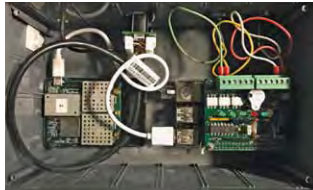
Figure 12-1. Prototype hardware for the next-generation SealD data logger, with enhanced GNSS capabilities. The GNSS receiver (left circuit board) records L1/L2 phase observables for post-processing; the data logger (right circuit boards) does preliminary pre-processing and stores the data, in addition to logging NMEA data from the observer’s navigational echosounder with minimal latency.
