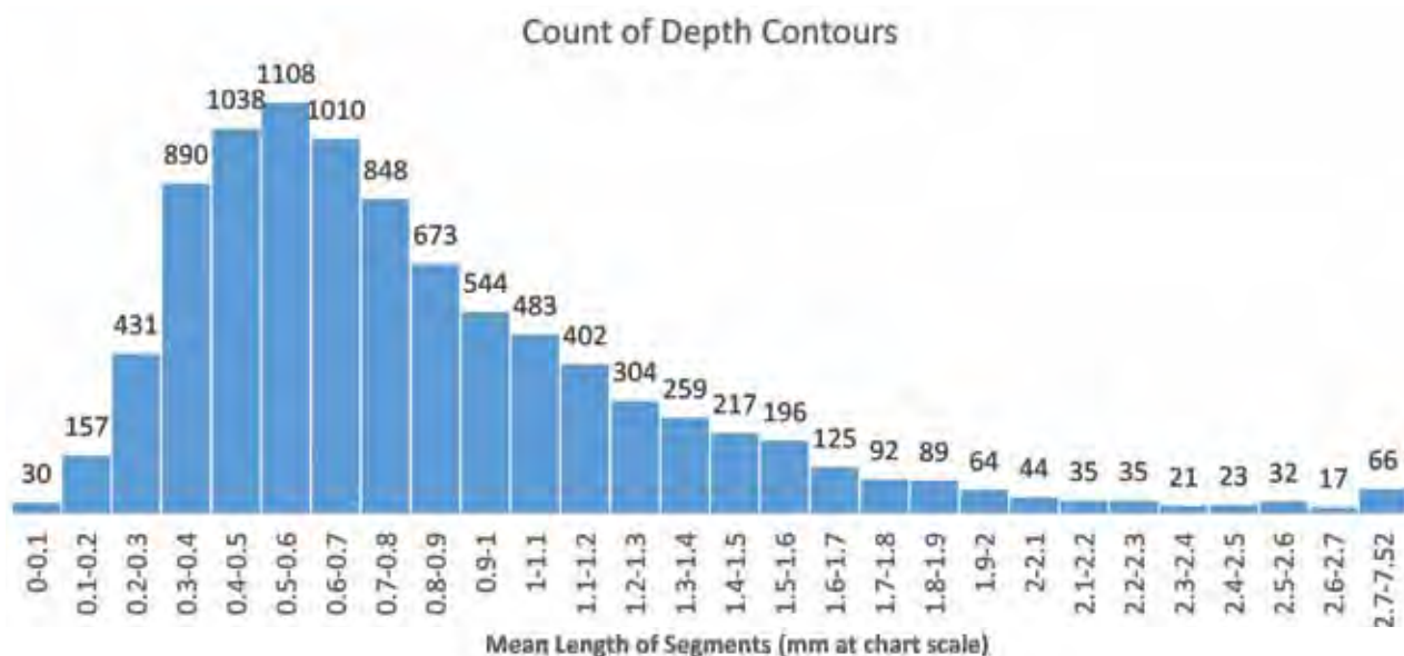
Figure 37-3. The histogram of the mean length of segments for contours with VALDCO 18.2m in ENC US5AK4DM. Data follow the exponentially modified Gaussian distribution with mean 0.82mm, standard deviation 0.51mm, kurtosis 10.52 and skewness 2.146.
