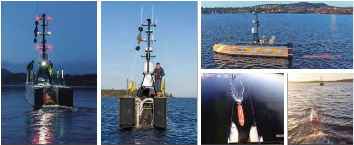
Figure 53-11. Images showing Launch and Recovery of the HUGIN AUV Chercheur on board the USV SEA-KIT Maxlimer . The vessel was named USV Maxlimer after one of GEBCO's alumna, Maxlimer Anziani Vallee, who was killed in a tragic accident on 24 January 2017 in Canada.
