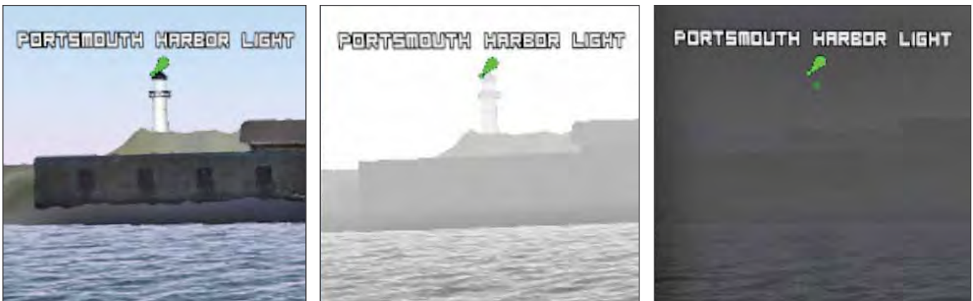
Figure 44-3. The AR marker over this lighthouse remains the same visually, across varied time-of-day and visibility conditions.
