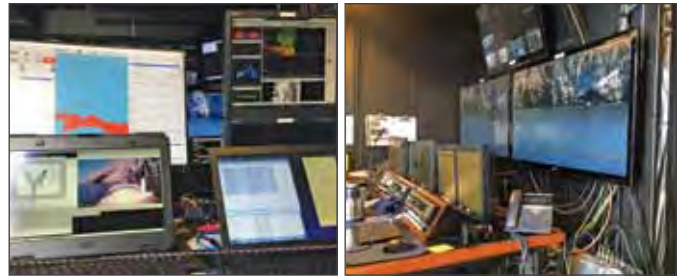
Figure 11-19. ASV operator's station (left) during survey along cliff walls of Santa Cruz Island, and the view of the ASV from the E/V Nautilus 's telephoto video system is shown above. Real time radar (overlay in red on the operator's top left map display) along with color and FLIR camera images allowed a remote operation of the ASV within 2 m of the cliff walls. Real time monitoring of data acquisition (upper right of operator's station) ensured quality and safe navigation.
