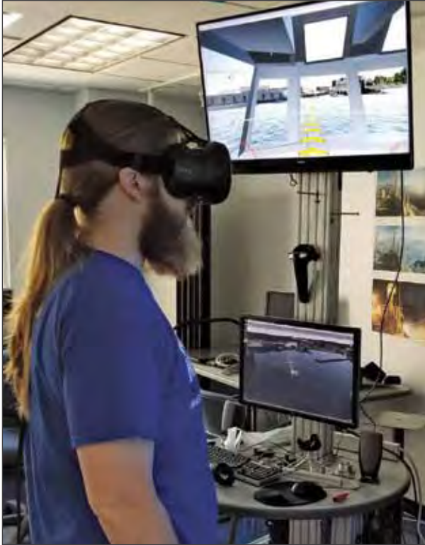
Figure 44-2. Using the VR-based AR simulator. Users wearing the head mounted display can walk around a virtual copy of the R/V Gulf Surveyor and see AR overlays, as mirrored in the monitor at the top of the photo.
