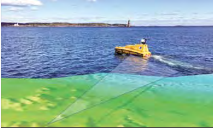
Figure I-17. BEN (Bathymetric Explorer and Navigator), the CWorker-4 model vehicle operating in the vicinity of Portsmouth Harbor, New Hampshire.
