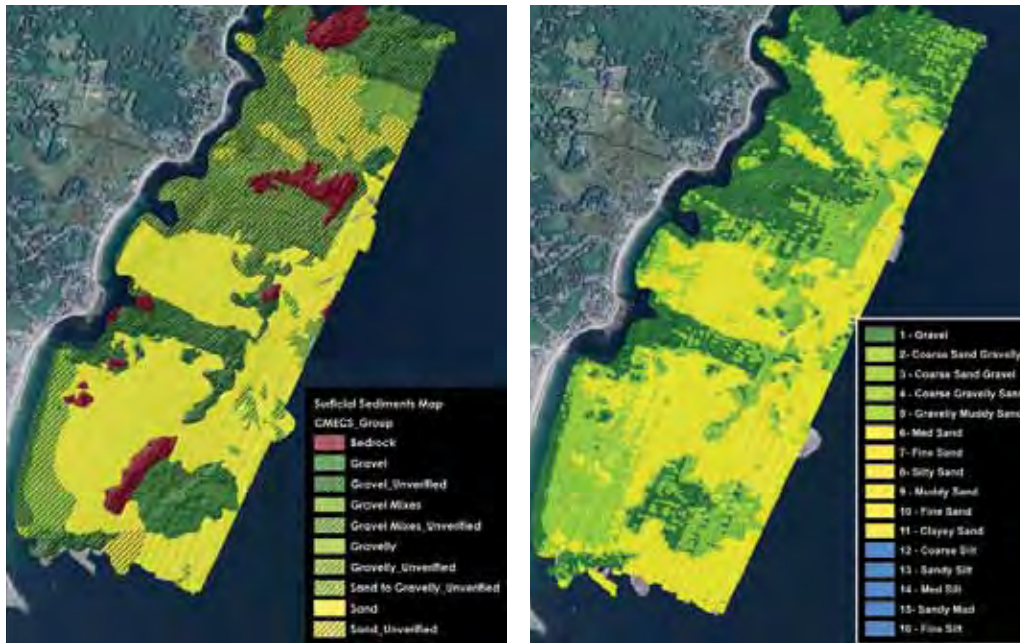
Figure 21-2. Example of Summer Hydro survey (SH 2015) where FMGT ARA was relatively successful in identifying bottom sediment type. Image on left is the CMECS map being used as ground truth. The map on the right is the results of the ARA. Note the seafloor types have been grouped into Gravel (dark green), gravel mixes (light green), sand mixes (yellow), and muddy mixes (blue). Crosshatched pattern on CMECS map indicates bottom type not verified. Although the ARA performed reasonably well here, the overall performance on a number of different surveys on the NH continental shelf was poor.
