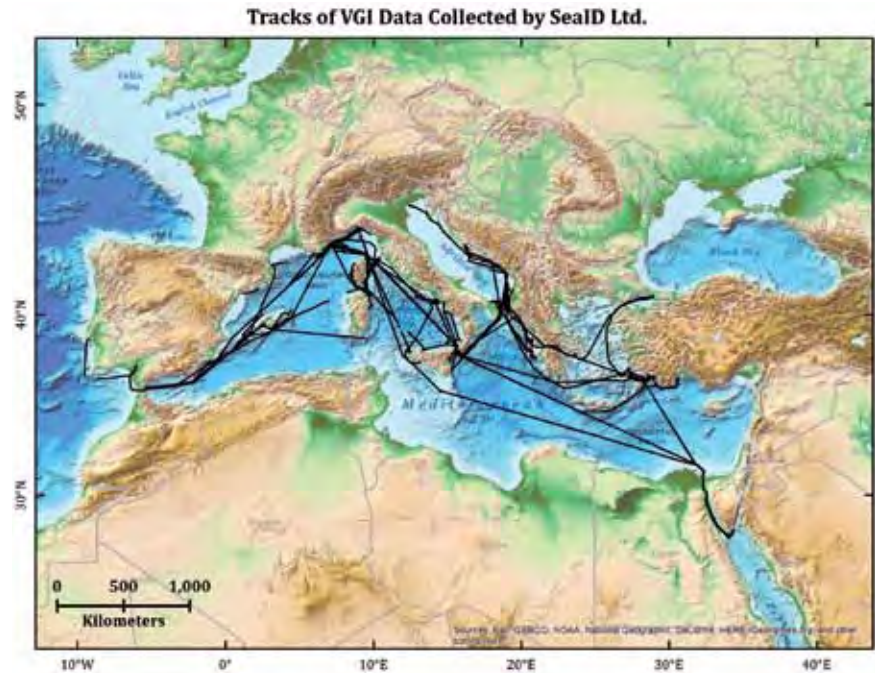
Figure 34.1. Example of tracklines from the SealD Ltd. database of volunteered geographical information collected from seven yachts in the Mediterranean Sea, parsed in Python and visualized as shapefiles in ArcGIS. Data of this type may provide depth information, but can also be useful simply for information about where ships go, and how frequently.
