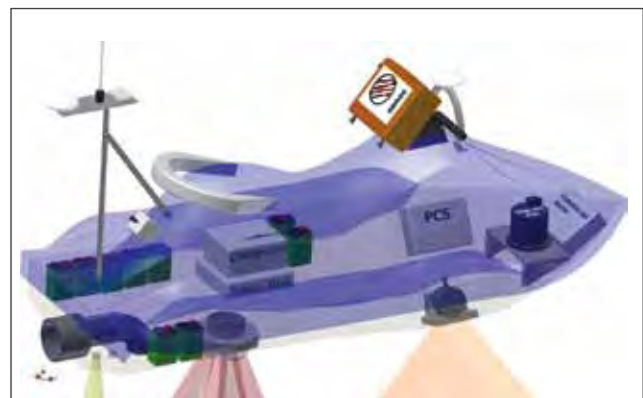
Figure I-14. CAD drawing of CBASS showing the location of the MBES peach), SBES (yellow), ADCP (red) with acoustic beam patterns on the CBASS. Also shown are the location of the POS MV IMU and PCS, onboard computers and LAN router, internal battery packs, GPS and RTK antennae, and navigational display monitor.
