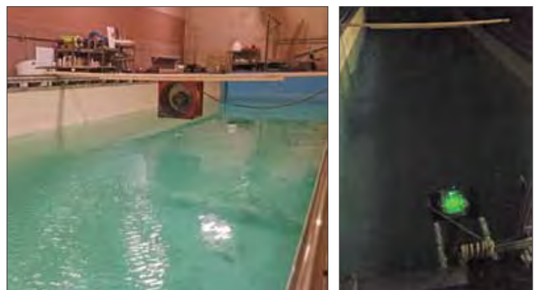
Figure 5-1. Water surface experimental setup. (Left) Fan mounted on the tow tank creates capillary surface waves. (Right) The optical detector array submerged underwater with the laser beam footprint. The incoming waves change the laser beam footprint location on the array.
