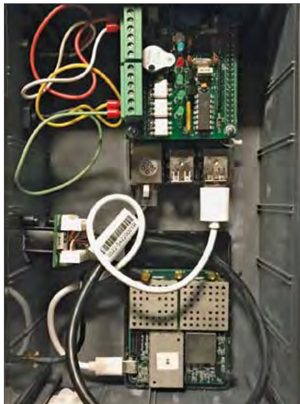
Figure ES-22. Prototype hardware for the next-generation SealD data logger, with enhanced GNSS capabilities. The GNSS receiver (bottom circuit board) records L1/L2 phase observables for post-processing; the data logger (top circuit boards) does preliminary pre-processing and stores the data, in addition to logging NMEA data from the observer’s navigational echosounder with minimal latency.
