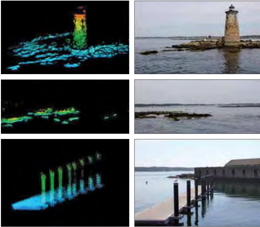
Figure 29-5. Shoreline features in Portsmouth Harbor as mapped by the Velodyne VLP-16 system during the July 2016 field experiments. Top : Whaleback lighthouse (70 m scanning range). Middle : Rocky islet (64 m scanning range). Bottom : Pilings and floating pier near Fort Point, NH.
