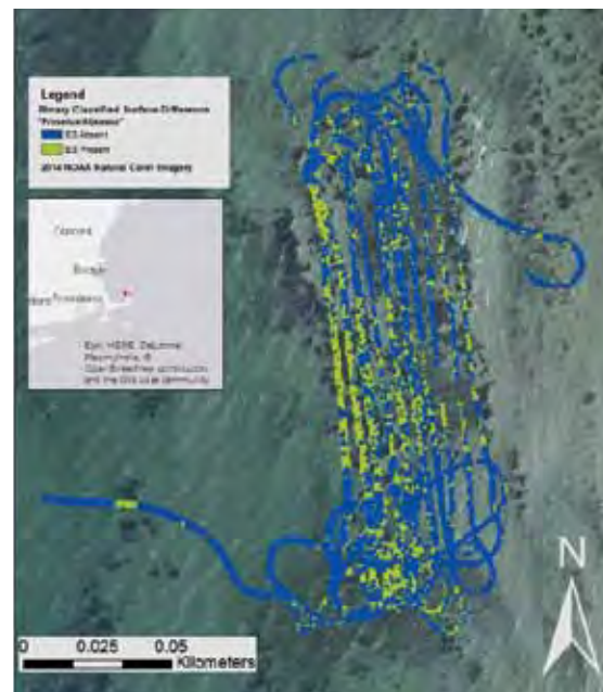
Figure 31-5. Binary-classified surface difference data from Duck Harbor, Cape Cod, MA, overlaid on NOAA low-tide aerial imagery.
