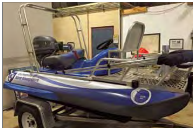
Figure I-16: The JHC Zego Boat, a highly maneuverable and stable twin-hulled catamaran that is being outfitted into a state-of-the-art shallow water survey vessel with MBES, SBES, and ADCP capabilities.
