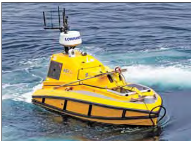
ES-11. ASV-BEN (left) and BEN and the Center's research vessel R/V Gulf Surveyor during survey and testing operations in Portsmouth Harbor (right).
