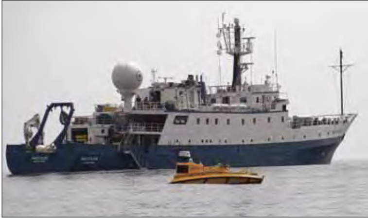
Figure ES-13. ASV-BEN deployed from the E/V Nautilus in July during mapping operations in the vicinity of the Channel Islands.
