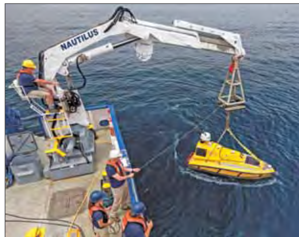
Figure 11-4. The newly designed lifting bail providing a single-point lift is shown in its stowed position on the ASV (left) and during vehicle retrieval operations (right). Photo by Ed McNichol, released under the Create Commons License ( http://creativecommons.org/licenses/by-nc-sa/4.0/ ). These photos have been cropped from their original size.
