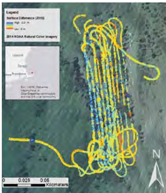
Figure 31-4. Surface difference between “canopy” and seafloor digital terrain models at Duck Harbor, Cape Cod, MA. Higher surface differences infer the presence of vegetation, and tend to overlay darker areas of vegetation in the aerial imagery as well.
