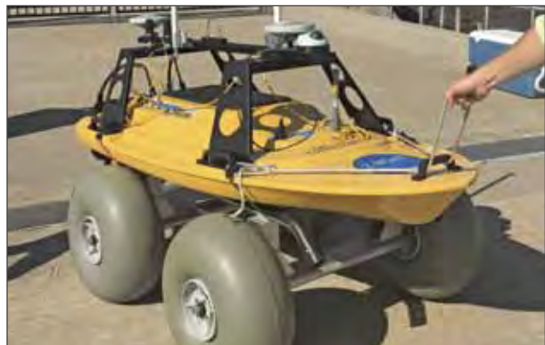
Figure I-18. The Teledyne OceanSciences "Z-boat" fitted to a wheeled cart typically used for jet-ski deployment from beaches.
