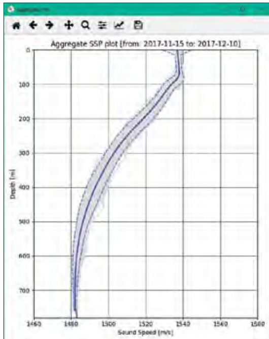
Figure 8-4. A SSM analysis tool to evaluate the variability of the collected sound speed profiles based on a user-selected temporal window. In this case, the profiles correspond to the survey shown in Figure 8-3.
