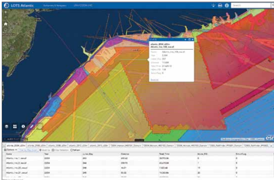
Figure 60-1. Atlantic Margin dynamic map web page distributed through the Center's website at https://ccom.unh.edu/gis/maps/Atlantic2017 . This interface allows users to view the Center's bathymetry and backscatter grids and query file names, survey domains, and depths from the Center's ECS holdings.
