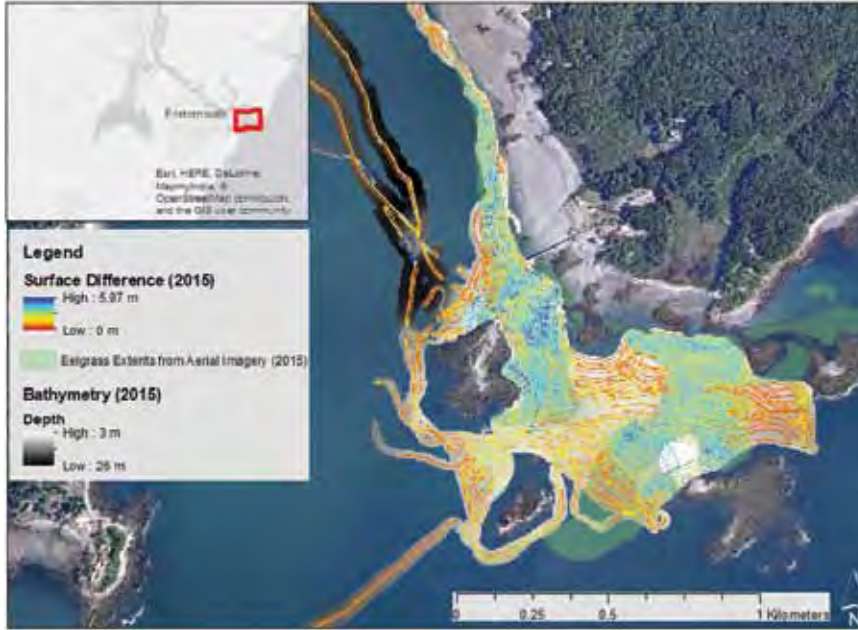
Figure 31-2. Surface difference between "canopy" and seafloor digital terrain models at Portsmouth Harbor, NH. Higher surface differences infer the presence of vegetation. Note that the borders of higher surface difference areas align well in shallow water, but not on the deeper edges.
