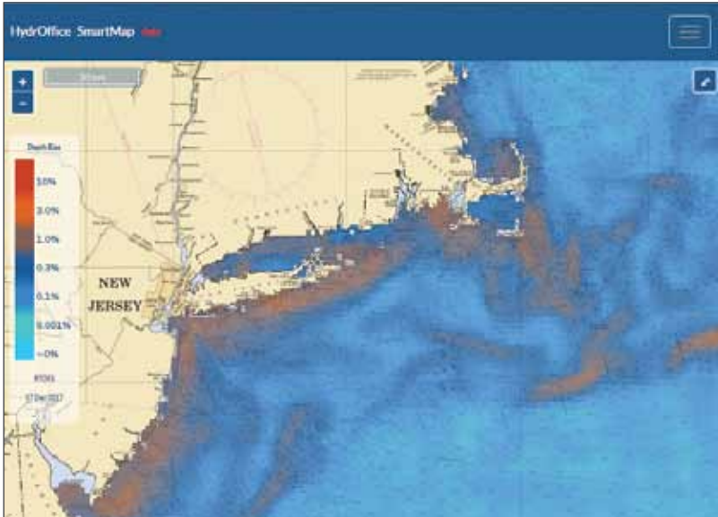
Figure ES-21. SmartMap visualization of global estimated ray-tracing uncertainty, expressed as depth bias, at 14 October 2017 based on the Global RTOFS-based 24-hr forecast (top) and detail view at 17 December 2017 (bottom). The depth bias percentage indicates where oceanographic variability is likely to cause higher or lower variability in acoustic ray tracing, allowing the surveyor to assess data quality issues that might ensue.
